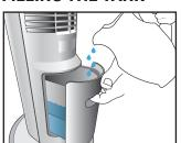
Pull out the drawer on the backside of the unit. Using a pitcher or other container, fill until MAX line. Be sure to at least fill until over MIN line or water pump will not function properly.
