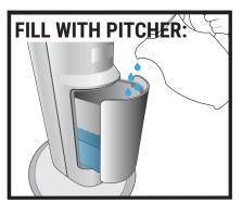
Place on flat surface & fill tank from a water pitcher. **For best results** use cold water and/or ice cubes.
