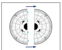
3. Align the assembled Base with the Arctic Air™ Tower. Pull the Power Cord through the hole in the center of the assembled Base.
