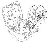
2. Install a new cutter unit. Push it in until it snaps into place.
