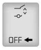
To change the liftgate to manual operation, press the switch on the center console to the OFF position.
