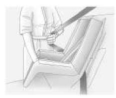
5. Pull the rest of the shoulder belt all the way out of the retractor to set the lock.
