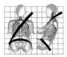
Sit up straight and always keep your feet on the floor in front of you. The lap part of the belt should be worn low and snug on the hips, just touching the thighs. In a crash, this applies force to the strong pelvic bones and you would be less likely to slide under the lap belt.
