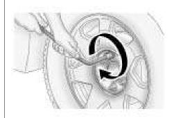
Loosen the wheel nuts — but do not remove them — using the lug wrench. For wheels with a wheel lock key, use the wheel lock key between the lock nut and lug wrench. The key is supplied in the front passenger door pocket. Notice: If this vehicle has wheel locks and an impact wrench is used to remove the wheel nuts, the lock nut or wheel lock key could be damaged. Do not use an impact wrench to remove the wheel nuts if this vehicle has wheel locks.
