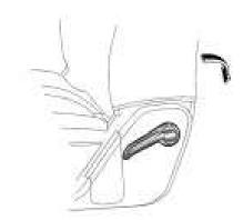
On vehicles with seats that have manual reclining seatbacks, the lever used to operate them is located on the outboard side of the seat.
