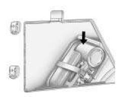
Press down on the latch tab and pull the cover off to access the storage compartment.
