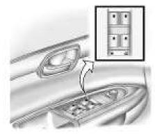
On vehicles with power windows, the switches are on the driver door armrest. Each passenger door has a switch that controls only that window.
