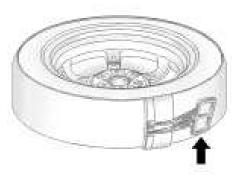
Remove the plastic spare tire heat shield by pulling the rubber latch. Store the plastic spare tire heat shield. See "Storing a Flat or Spare Tire and Tools" later in this section for more information.
