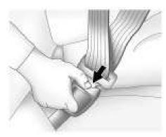
To unlatch the belt, push the button on the buckle. The belt should return to its stowed position. Slide the latch plate up the safety belt webbing when the safety belt is not in use. The latch plate should rest on the stitching on the safety belt, near the guide loop on the side wall.
