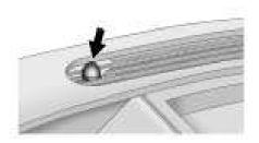
The solar sensor, located in the defrost grille in the middle of the instrument panel, monitors the solar heat. Do not cover the solar sensor or the system will not work properly.
