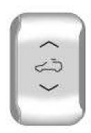
The switch to operate the front sunroof is on the headliner above the rearriew mirror.
