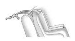
If the position you are using does not have a headrest or head restraint and you are using a dual tether, route the tether over the seatback.
