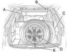
4. Pull the cable (A) through the door striker (E), the center of the wheel (D), and the plastic spare tire heat shield (C), as shown.
