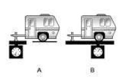
If a weight-carrying hitch or a weight-distributing hitch is being used, the trailer tongue (A) should weigh 10-15 percent of the total loaded trailer weight (B).
