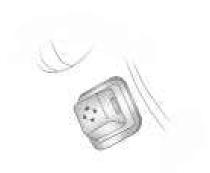
For vehicles with the power tilt and telescope wheel, the control is on the left side of the steering column.
