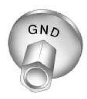
Connect the other end of the negative (-) cable at least 18 inches (45 cm) away from the dead battery, but not near engine parts that move.
