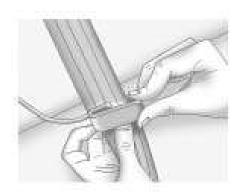
2. Place the guide over the belt and insert the two edges of the belt into the slots of the guide.
