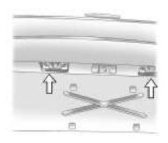
2. Turn and pull the license plate lamp forward through the lift gate trim opening.
