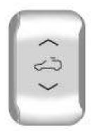
**Vent:** From the closed position, press and hold the front of the switch to vent the sunroof. Press and hold the rear of the switch to close the sunroof.
