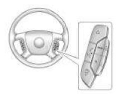
$\triangle$  /  $\nabla$ : Press to change favorite radio stations, select tracks on a CD/DVD, or to navigate tracks or folders on an iPod<sup>®</sup> or USB device.
