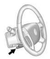
Pull the lever down to move the steering wheel up or down and in or out. Pull the lever up to lock the steering wheel in place.
