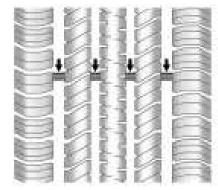
One way to tell when it is time for new tires is to check the treadwear indicators, which appear when the tires have only 1.6 mm (1/16 inch) or less of tread remaining. The vehicle needs new tires if any of the following statements are true:
