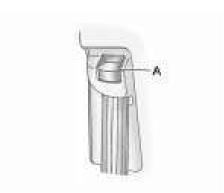
To move it down, push down on the button (A) and move the height adjuster to the desired position. You can move the height adjuster up by pushing up on the shoulder belt guide.
