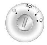
The ignition switch has four different positions.
