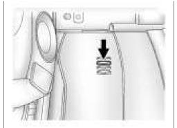
The interior temperature sensor located on the instrument panel to the right of the steering column, measures the temperature of the air inside the vehicle.
