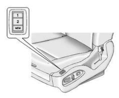
On vehicles with the memory feature, the "1" and "2" buttons on the outboard side of the driver seat are used to manually save and recall the positions of the driver seat, outside mirrors, and adjustable throttle and brake pedal positions, if available. These manually stored positions are referred to as Button Memory positions.
