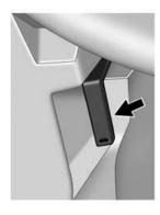
1. Pull the release handle with the above symbol on it. It is located below the instrument panel to the left of the steering wheel.
