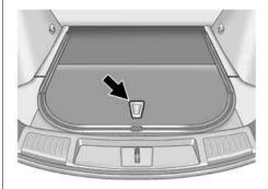
To open the cargo management system, press the handle to unlatch and then lift up.
