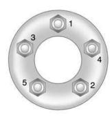
16. Tighten the wheel nuts firmly in a crisscross sequence, as shown.
