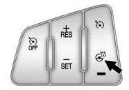
For vehicles with a heated steering wheel, the button for this feature is located on the steering wheel.
