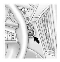
The vehicle has an electronic keyless ignition with pushbutton start.
