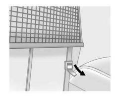
6. Pull on the straps to tighten the net.
