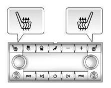
If available, the buttons are on the Rear Sear Audio (RSA) panel on the rear of the center console.
