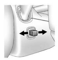
The switch used to adjust the pedals is located on the right side of the steering column, below the wiper stalk.
