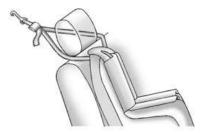
If you are using a dual tether in the rear outboard seating position with an adjustable head restraint, route the dual tether around the head restraint.
