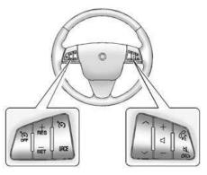
Use these controls, if equipped, to make audio adjustments at the steering wheel.
