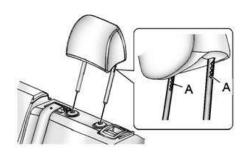
Insert the head restraint posts into the holes in the top of the seatback. The notches (A) on the posts must face the driver side of the vehicle.  Push the head restraint down.
