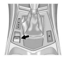
The vehicle has an Electric Parking Brake (EPB). The switch for the EPB is in the center console. The EPB can always be activated, even if the ignition is off. To avoid draining the battery, do not cycle the EPB too often without the engine running. The EPB can be left applied while the vehicle is parked.
