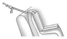
If you are using a single tether in the rear outboard seating position and the head restraint has been removed, route the single tether over the seatback.
