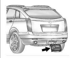
The vehicle may have a hitch cover. To remove the hitch cover:
