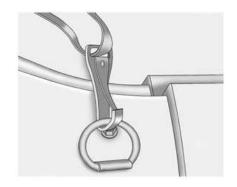
5. Attach the strap to the cargo tie-down in the rear of the vehicle.
