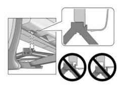
Raise the vehicle by turning the wheel wrench clockwise until the slots in the jack head fit into the metal flange located behind the triangle on the plastic moulding.
