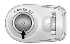
The front fog lamp button is located on the exterior lamp control, on the outboard side of the steering wheel.
