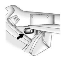
The glove box is air conditioned and can be used to store items at a lower temperature. The vehicle air conditioning must be turned on for the maximum cool air to enter the glove box.
