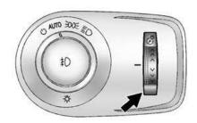
This feature controls the brightness of the instrument panel lights.
