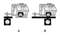
If a weight-carrying hitch or a weight-distributing hitch is being used, the trailer tongue (A) should weigh 10-15 percent of the total loaded trailer weight (B).
