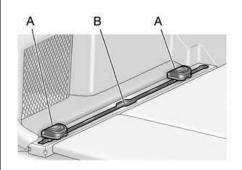
Insert the D-ring sliders (A) into the channel (B) located in the middle of the rail. Push the button to move the D-ring slider along the rail.
