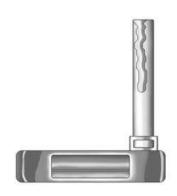
This key, located inside the Remote Keyless Entry (RKE) transmitter, is used for the driver door and glove box.
