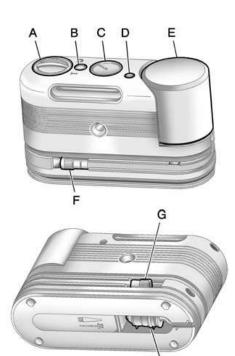
When using the tire sealant and compressor kit during cold temperatures, warm the kit in a heated environment for five minutes. This will help to inflate the tire faster.
