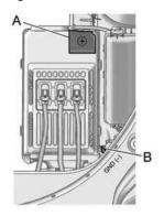
Your vehicle is equipped with a remote positive (+) terminal (A) and a remote negative (-) terminal (B).
