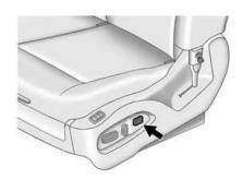
If available, press and hold the front or rear of the control to increase or decrease lumbar support. Release the control when the seatback reaches the desired level of lumbar support.
