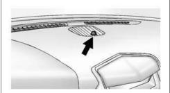
This feature automatically turns the lamps on and off. A light sensor on top of the instrument panel makes the Twilight Sentinel® work, so be sure it is not covered.
