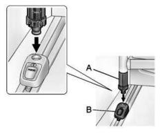
Push both adapter buttons to move the adapters (B) on the straight part of the u-rail.
