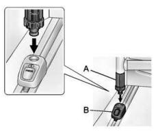
Insert the fence into the adapters and lock both latches (A) by turning to align  $\bigcirc$  with the arrow on the adapter (B).
