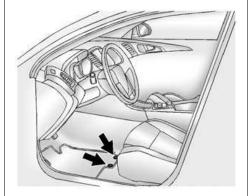
Pull up on the rear of the floor mat to unlock each retainer and remove.
