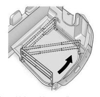
For vehicles with a u-rail system, the fence can be moved to different positions on the u-rail track to secure cargo.
