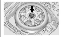
4. Remove the nut retaining the spare tire.
