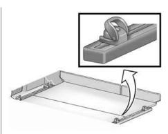
The loop of the D-ring slider must be facing inward toward the storage area and the ring must be in the up position for proper usage.
