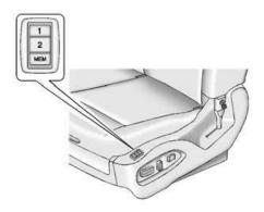
On vehicles with the memory feature, the "1" and "2" buttons on the outboard side of the driver seat are used to manually save and recall the positions of the driver seat, outside mirrors, and adjustable throttle and brake pedals, if available. These manually stored positions are referred to as Button Memory positions.
