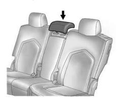
The vehicle's rear seat has an adjustable headrest in the center seating position that can be adjusted the same way as the outboard head restraints.
