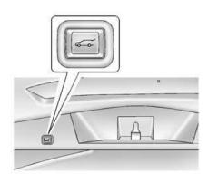
Press and release on the liftgate next to the latch to close the liftgate.
