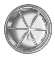
From the back side of the headlamp assembly, remove the top cap to replace the low-beam headlamp/DRL bulb.
