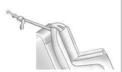
If you are using a single tether in the rear center seating position, lower the adjustable headrest down to its stowed position and route the single tether over the headrest. 3. Before placing a child in the child restraint, make sure it is securely held in place. To check, grasp the child restraint at the LATCH path and attempt to move it side-to-side and back-and-forth. There should be no more than 2.5 cm (1 in) of movement for proper installation.
