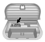
This vehicle may have a tire sealant and compressor kit in place of a jack or spare tire. It is located in a foam container in the rear compartment storage area. If the vehicle has a cargo cover, see Cargo Management System on page 4-4 for instructions on how to access the tire sealant and compressor kit.
