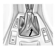
2. Remove the shift lever boot by pulling up on the rear of the trim plate.
