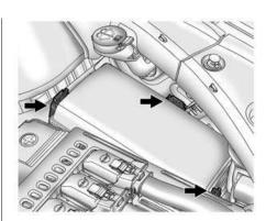
Unlatch three clips and lift up the underhood electrical center cover to remove.
