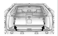
5. Mount the cargo net to the cargo tie-downs located on the lower side panels.
