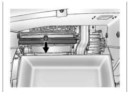
Release the two latches holding the service door. Lower the service door.
