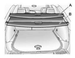
The shade can be set in two positions. It can be set in a halfway open (A) position for loading objects
