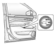
On vehicles with a power liftgate, the switch is on the driver door. The vehicle must be in P (Park) to use the power feature. The taillamps flash when the power liftgate moves.
