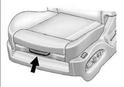
If available, adjust the manual leg extension by pulling up on the lever, and then pulling or pushing on the support to lengthen or shorten it. Release the lever to lock it in place.
