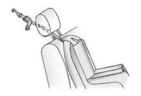
If you are using a single tether in the rear outboard seating position with an adjustable head restraint, route the single tether under the head restraint and in between the head restraint posts.
