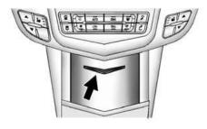
A storage area is located in front of the shift lever. Push upward on the top of the door and release; the door automatically opens.
