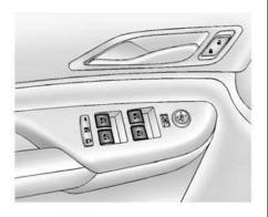
Pushing or pulling the switch part of the way will open or close the window as long as the switch is operated.
