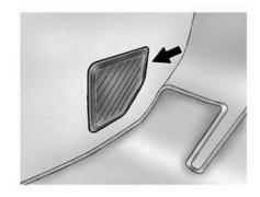
The instrument panel fuse block is located in the center console between the driver and passenger seats. To access the fuses, open the fuse panel door from the passenger side by pulling it out.
