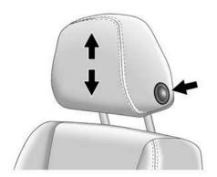
The height of the head restraint can be adjusted. To raise or lower the head restraint, press the button located on the side of the head restraint, and pull up or push the head restraint down, and release the button. Pull and push on the head restraint after the button is released to make sure that it is locked in place.
