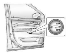
On vehicles with a power liftgate the switch is located on the driver door. The vehicle must be in P (Park) to use the power feature. The taillamps flash when the power liftgate moves.
