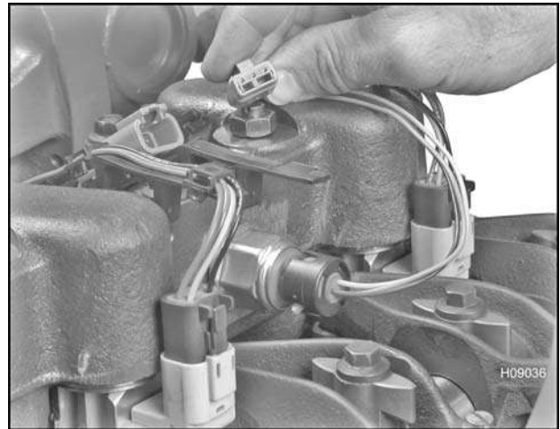
Figure 482 Disconnecting the BCP sensor
