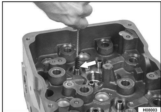
Figure 162 Cleaning valve guides
