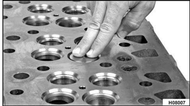
Figure 173 Turning valve on valve seat
