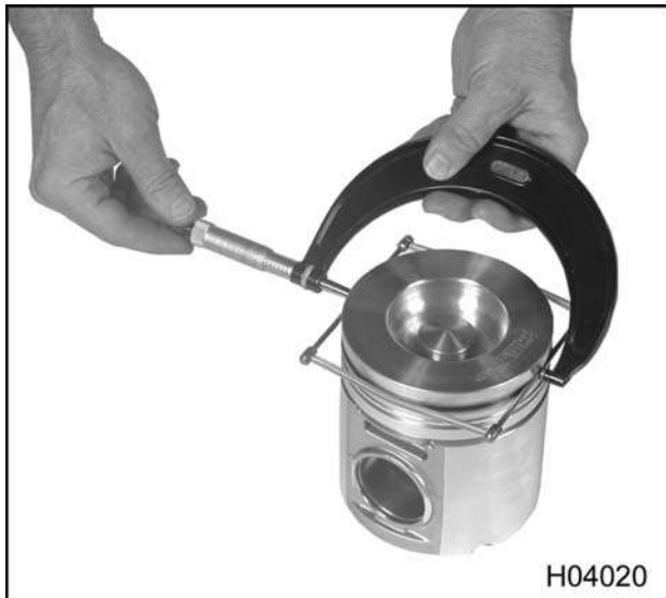
Figure 310 Measuring ring grooves with piston ring gauge pins
