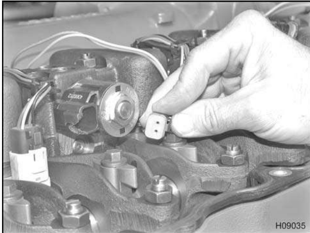
Figure 622 Disconnecting brake shutoff valve
