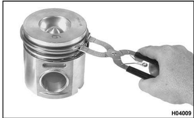
Figure 308 Removing piston rings (DT 466 piston shown)
