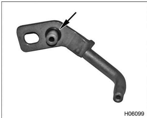
Figure 357 O-ring (underside) of new piston cooling tube
