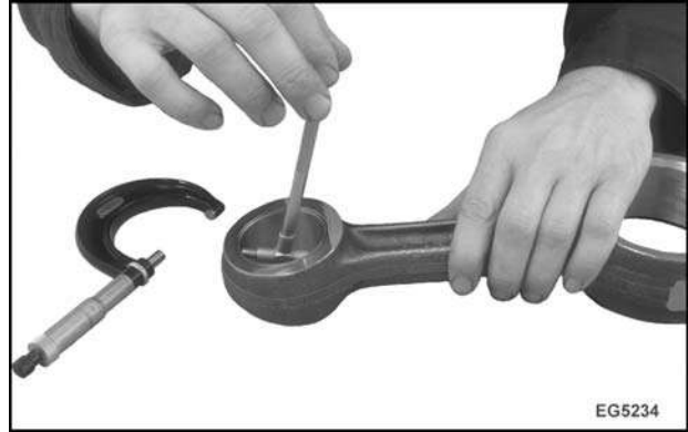
Figure 315 Measuring piston pin bushing inside diameter
