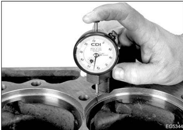
Figure 325 Checking counterbore depth with surface gauge
