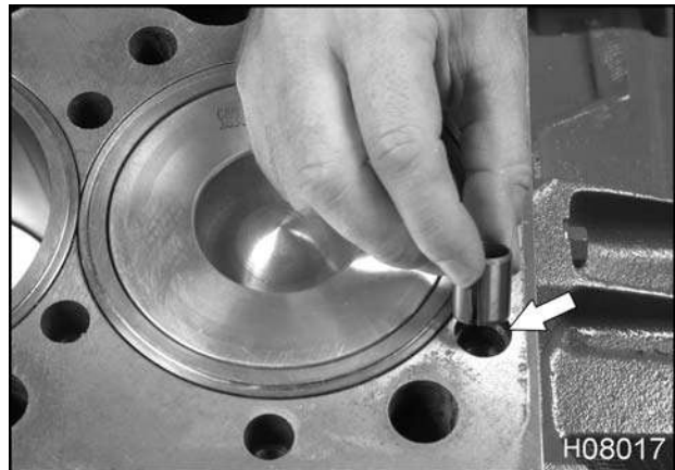
Figure 195 Installing alignment dowels
