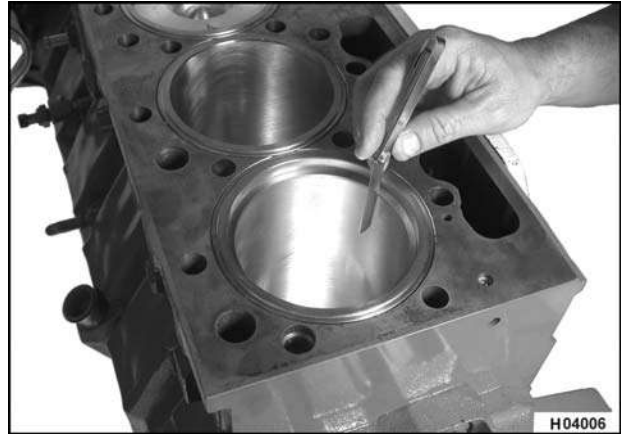
Figure 324 Checking cylinder sleeve piston ring end gap
