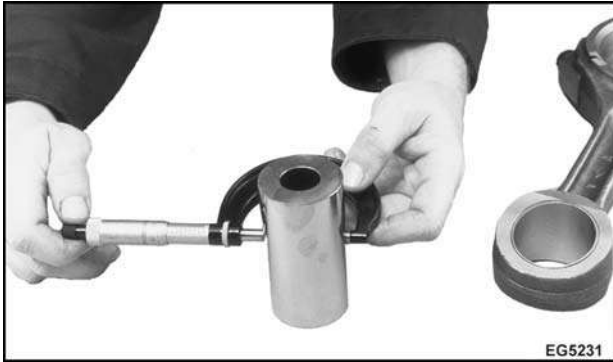
Figure 314 Measuring piston pin outside diameter
