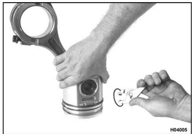
Figure 305 Removing piston pin retaining rings
