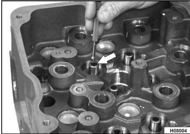
Figure 163 Measuring valve guide with ball gauge
