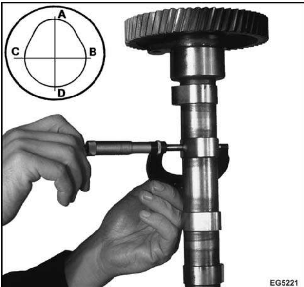
Figure 140 Measuring cam lobes with micrometer
