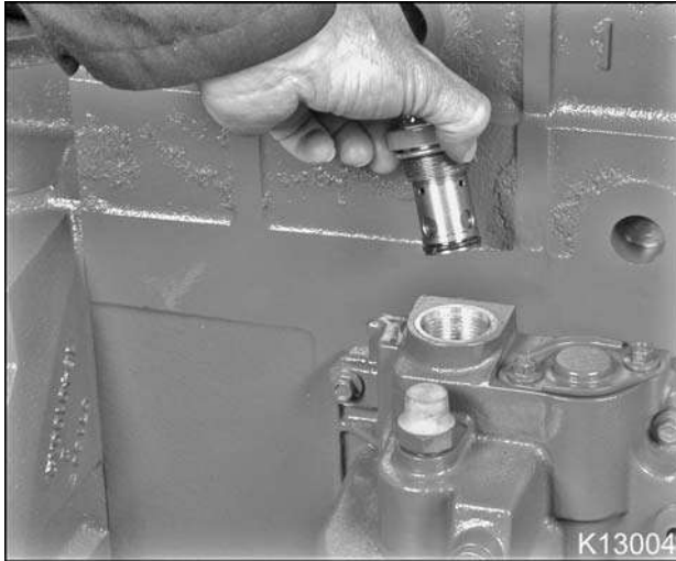
Figure 413 Removing the regulating valve
