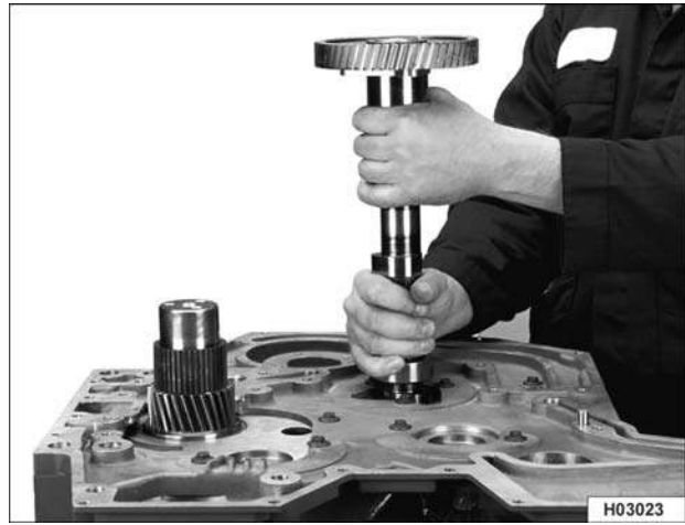
Figure 382 Installing camshaft assembly
