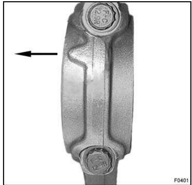
Figure 348 Connecting rod cap with M12 connecting rod cap bolts (protrusion points to front of engine)
