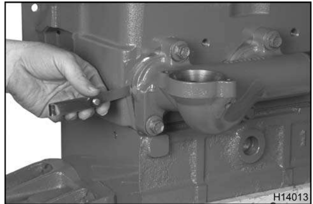
Figure 75 Checking exhaust manifold for cracks and warpage
