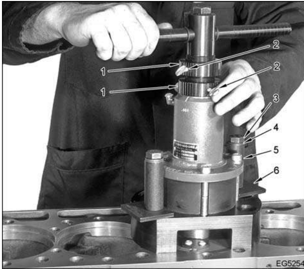
Figure 333 Positioning counterboring tool
