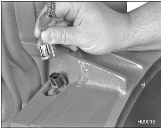
Figure 464 Disconnecting the CKP sensor
