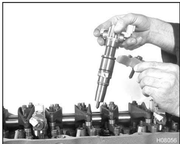
Figure 548 Removing the fuel injector assembly
