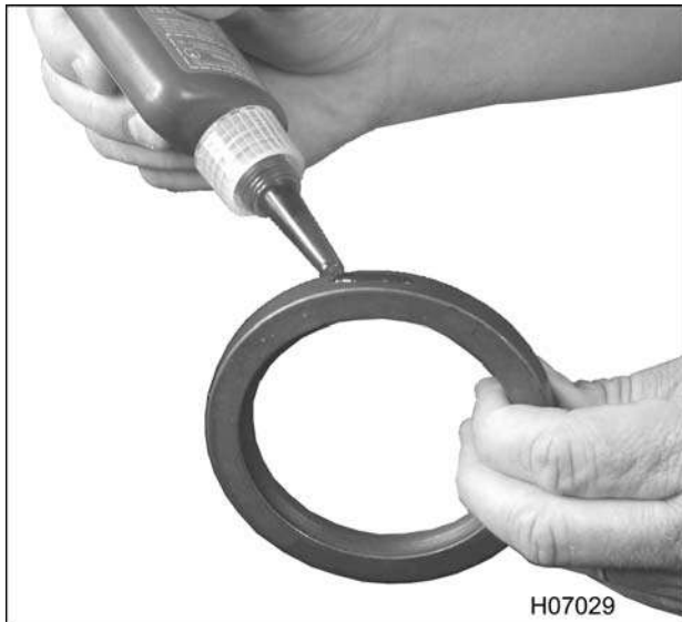
Figure 257 Applying Loctite® hydraulic sealant to front oil seal
