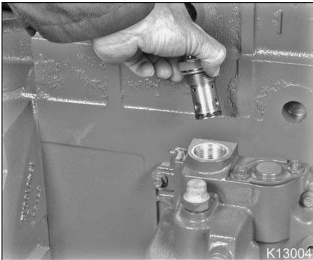
Figure 429 Installing the oil pressure regulating valve
