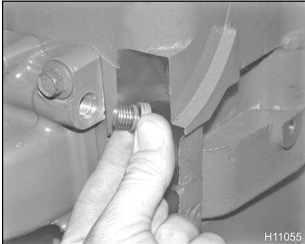
Figure 571 Installing the fuel rail plug assembly (2)
