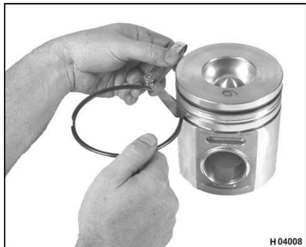
Figure 311 Measuring side clearance of oil control ring groove
