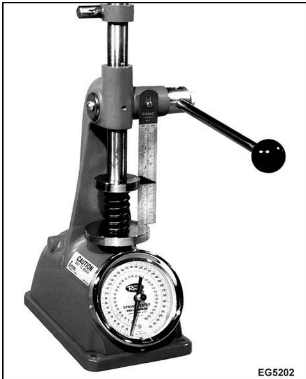
Figure 186 Measuring valve spring tension
