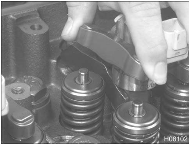
Figure 139 Removing the valve bridge
