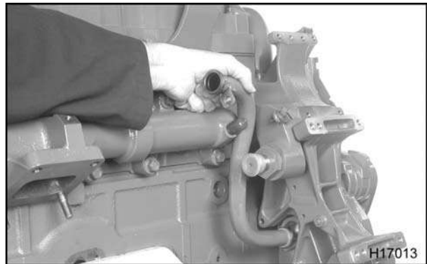
Figure 101 EGR cooler supply tube
