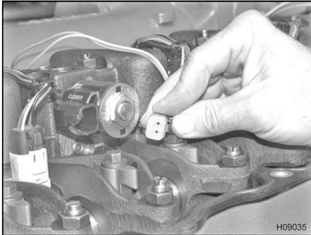
Figure 488 Connecting brake shutoff valve
