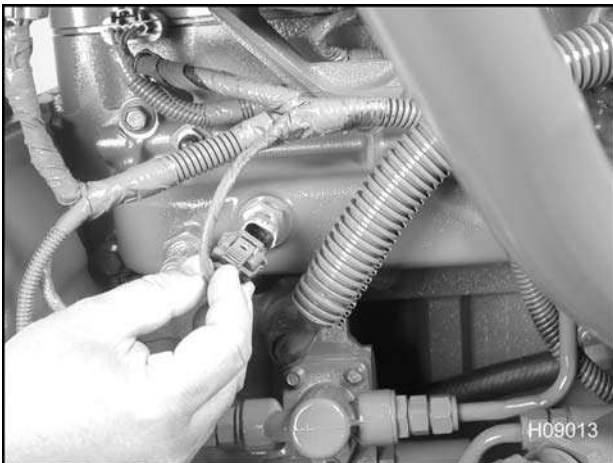
Figure 457 Disconnecting the MAT sensor
