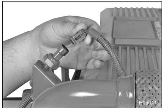
Figure 516 Connecting to the EBP sensor
