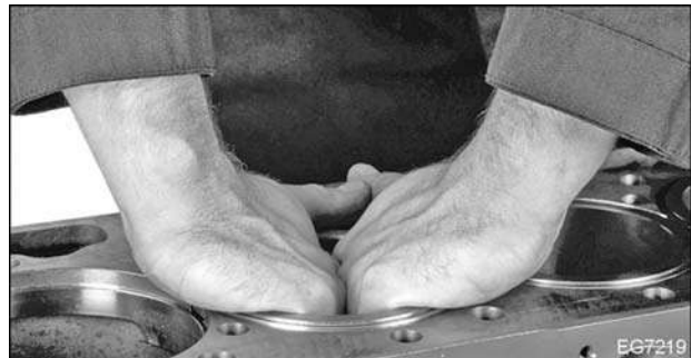
Figure 336 Installation of cylinder sleeve
