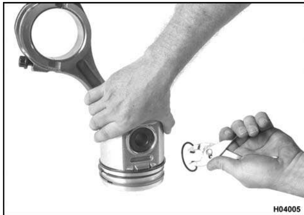
Figure 343 Installing piston pin retaining rings
