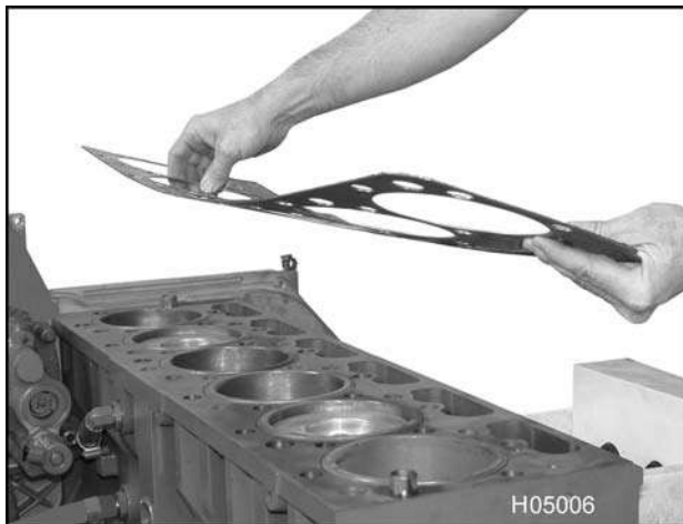
Figure 145 Removing cylinder head gasket
