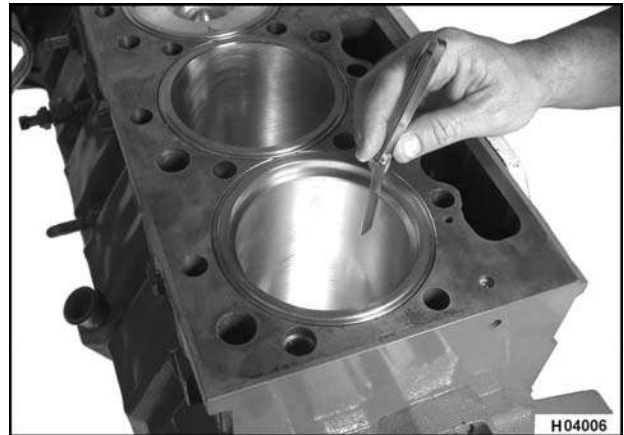
Figure 313 Checking piston ring end gap
