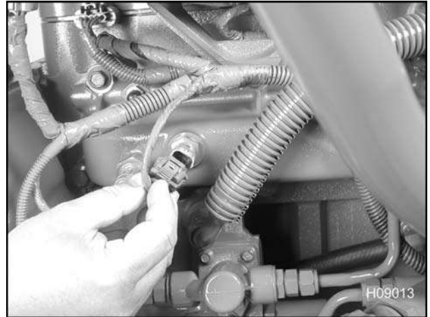
Figure 512 Connecting to the MAT sensor
