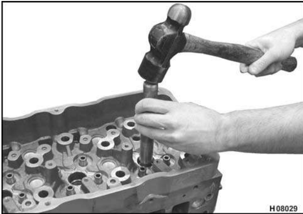
Figure 191 Installing fuel injector sleeve
