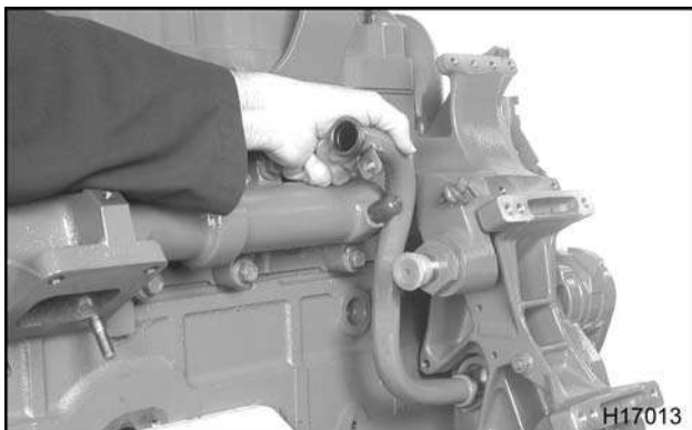
Figure 103 EGR cooler supply tube
