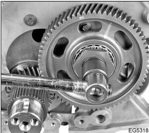
Figure 236 Removing the lower idler gear
