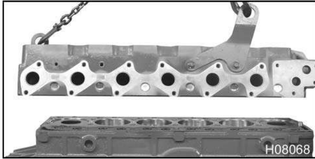
Figure 144 Removing cylinder head from crankcase
