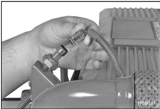
Figure 453 Disconnecting the EBP sensor
