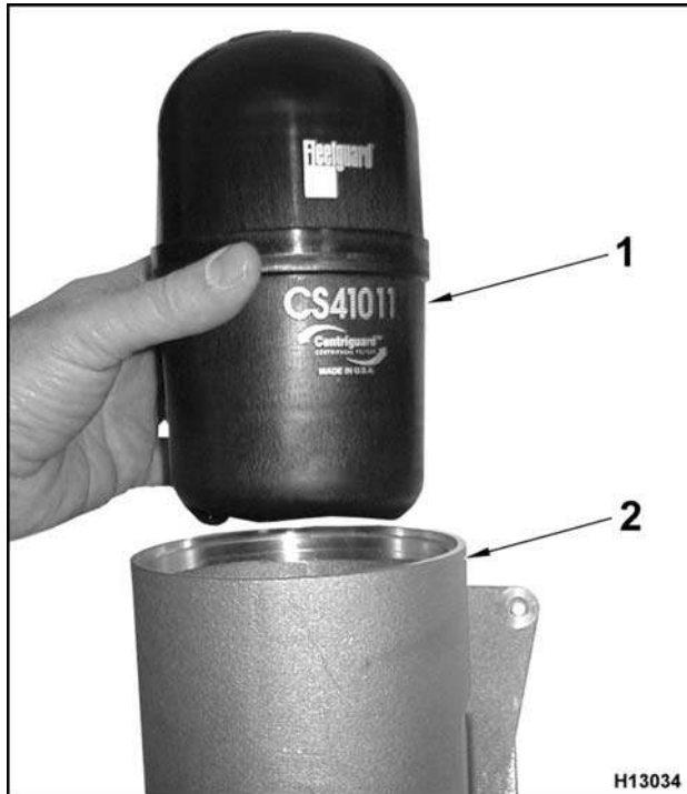
Figure 432 Secondary filter installation
