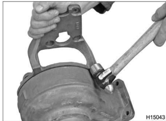
Figure 6 Removal of actuator flange
