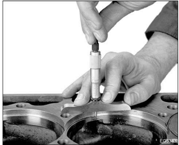
Figure 326 Checking counterbore depth with depth micrometer
