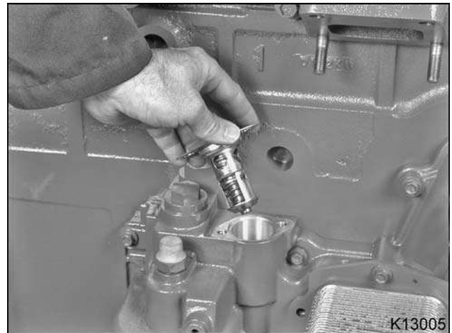
Figure 428 Installing the oil thermal valve
