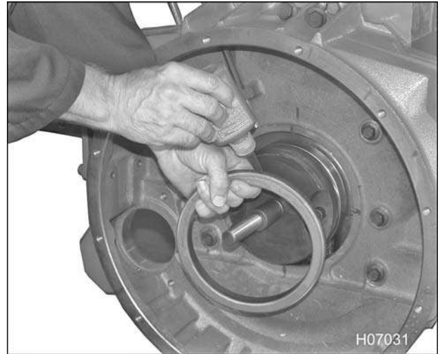
Figure 605 Applying sealant to the seal assembly
