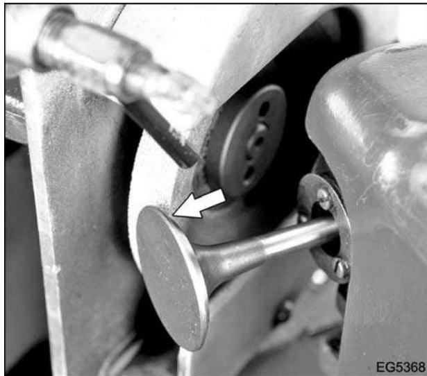
Figure 168 Grinding valve face
