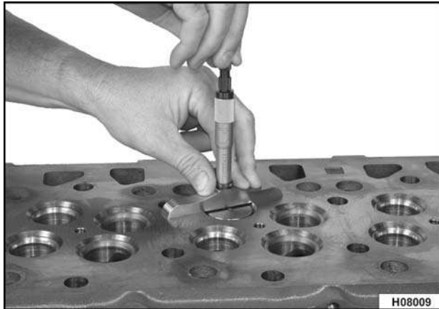
Figure 177 Checking valve recession
