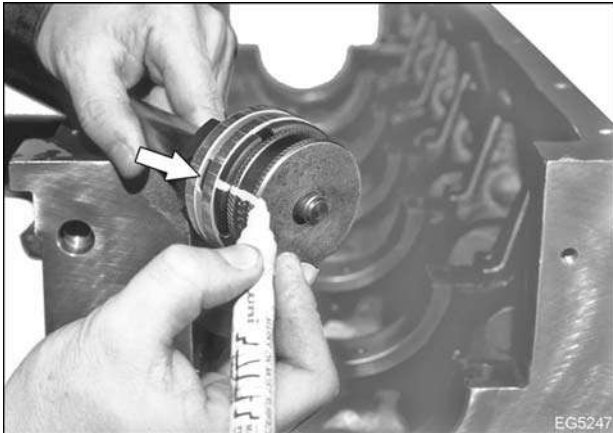
Figure 378 Marking oil hole location on bushing
