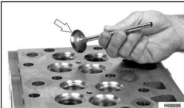
Figure 172 Applying Prussian Blue® to valve face
