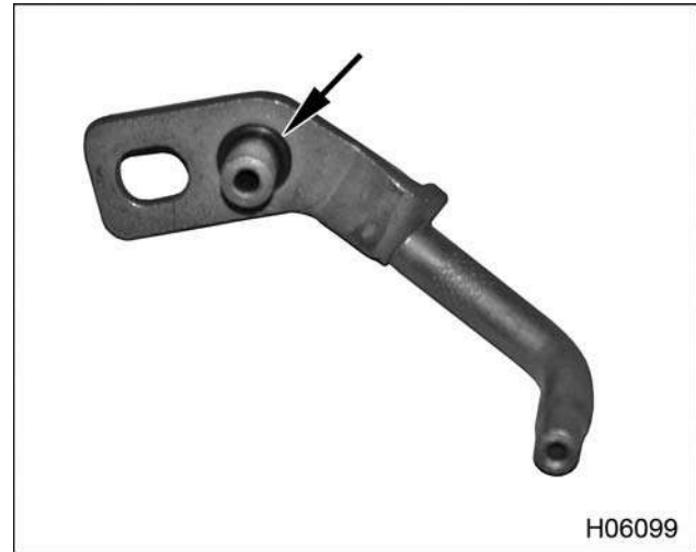
Figure 300 O-ring (underside) of new piston cooling tube
