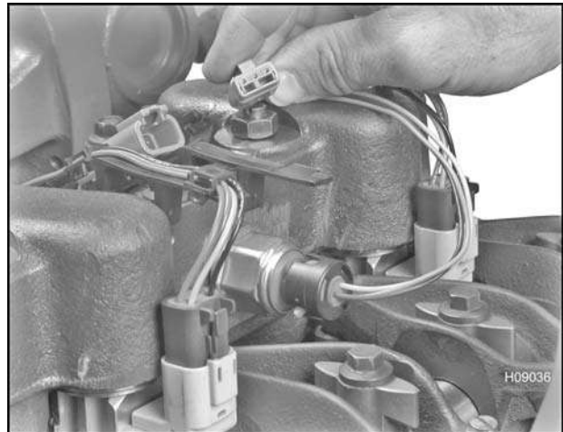
Figure 487 Connecting the BCP sensor
