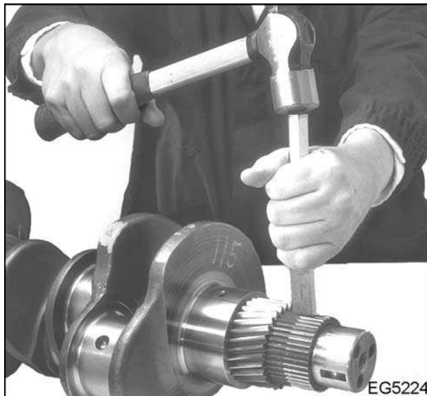
Figure 367 Removing oil pump drive spline
