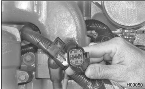
Figure 466 12 wire engine connector
