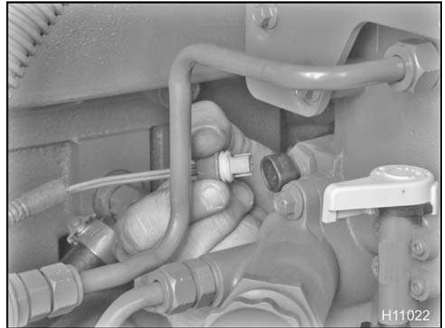
Figure 463 Disconnecting the WIF sensor
