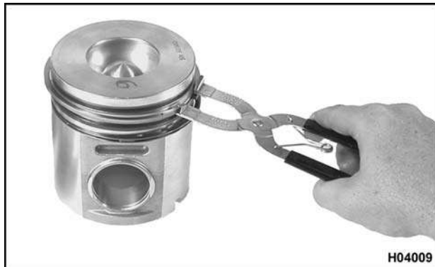
Figure 337 Installing piston rings (466 piston shown)
