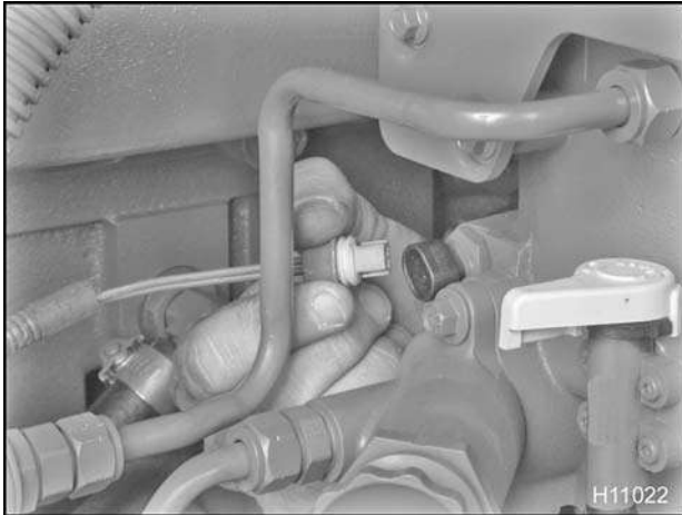
Figure 506 Connecting to the WIF sensor
