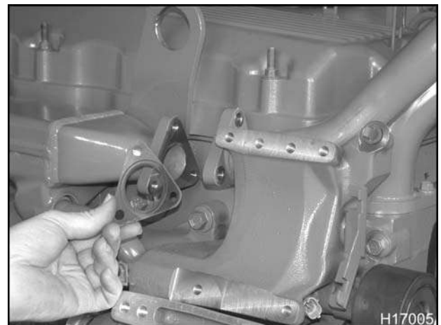
Figure 90 Removing the gasket
