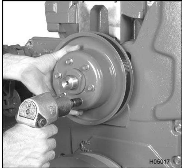
Figure 219 Removing the fan drive pulley
