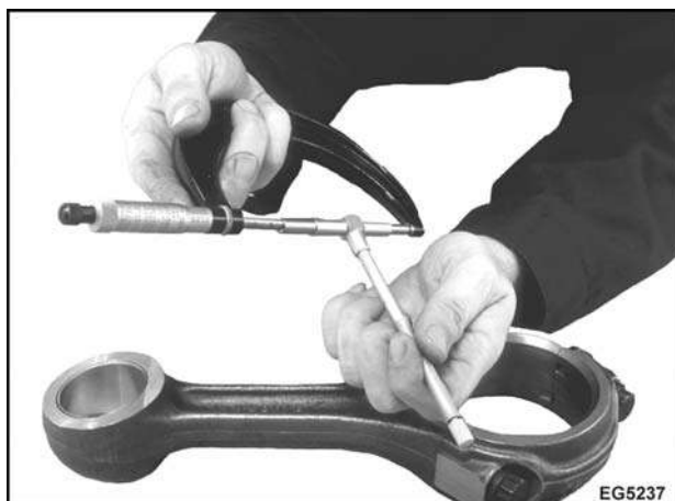
Figure 317 Measuring connecting rod bearing bore taper
