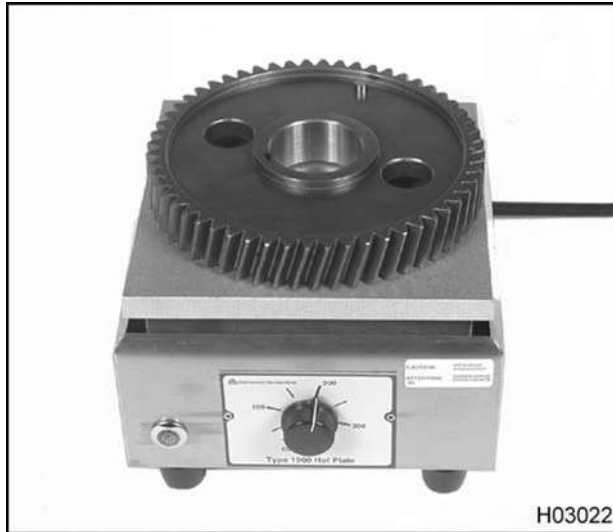
Figure 384 Heating the camshaft gear
