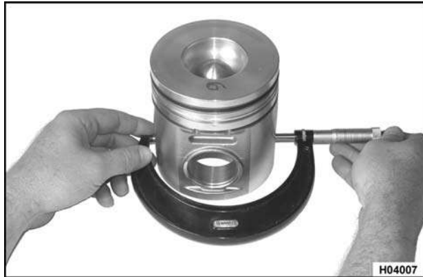
Figure 312 Measuring piston skirt diameter
