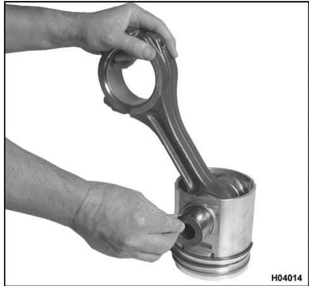
Figure 340 Installing piston pin
