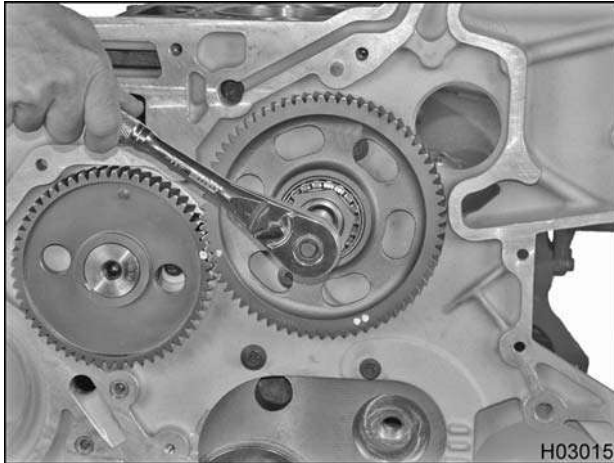
Figure 238 Removing the upper idler gear
