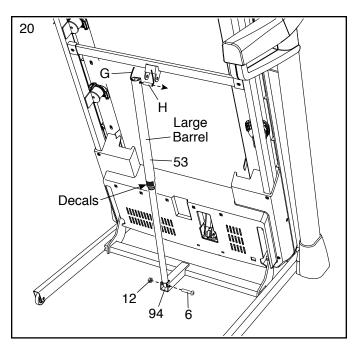
Attach the upper end of the Storage Latch (53) to the bracket on the Latch Crossbar (38) with a 5/16" x 2 1/4" Bolt (3) and a 5/16" Nut (12).
