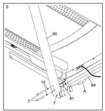
Remove the four indicated 5/16" x 3/4" Screws (4) from the Uprights (89, 90) (only one side is shown). The Screws will be used in a later step.
