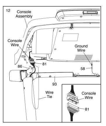
Set the console assembly on the brackets on the Handrails (86). Make sure not to pinch any wires. Insert the excess Upright Wire (81) into the Right Upright (90).
