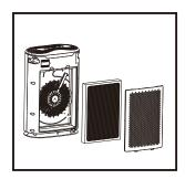
5. Remove all packages of filters, then install the new ones into the air purifier orderly.
