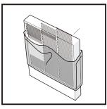
To reinstall the back cove, please align at the fixed groove and insert the cover into the groove, making the play button and frame withhold.
