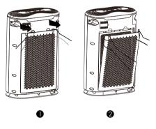
3. Disassemble all the filters.
