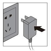
Plug the air purifier into a powered electrical outlet. The unit will set out a sound and all the indicators will be on. Then the power light will flash to enter the standby mode.
