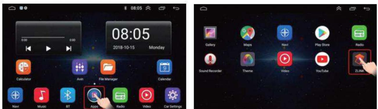
(2) Connect the original data cable of your mobile phone to the mobile phone, and plug the other end into the USB port of the MP5 car player (Note: Please use 4pin USB cable to connect)
