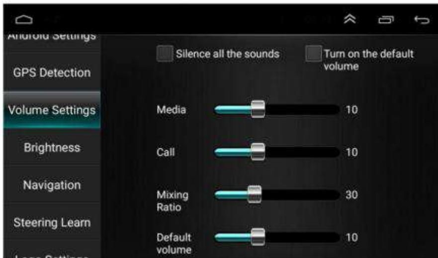
Users can adjust the volume ratio in different mode here.
