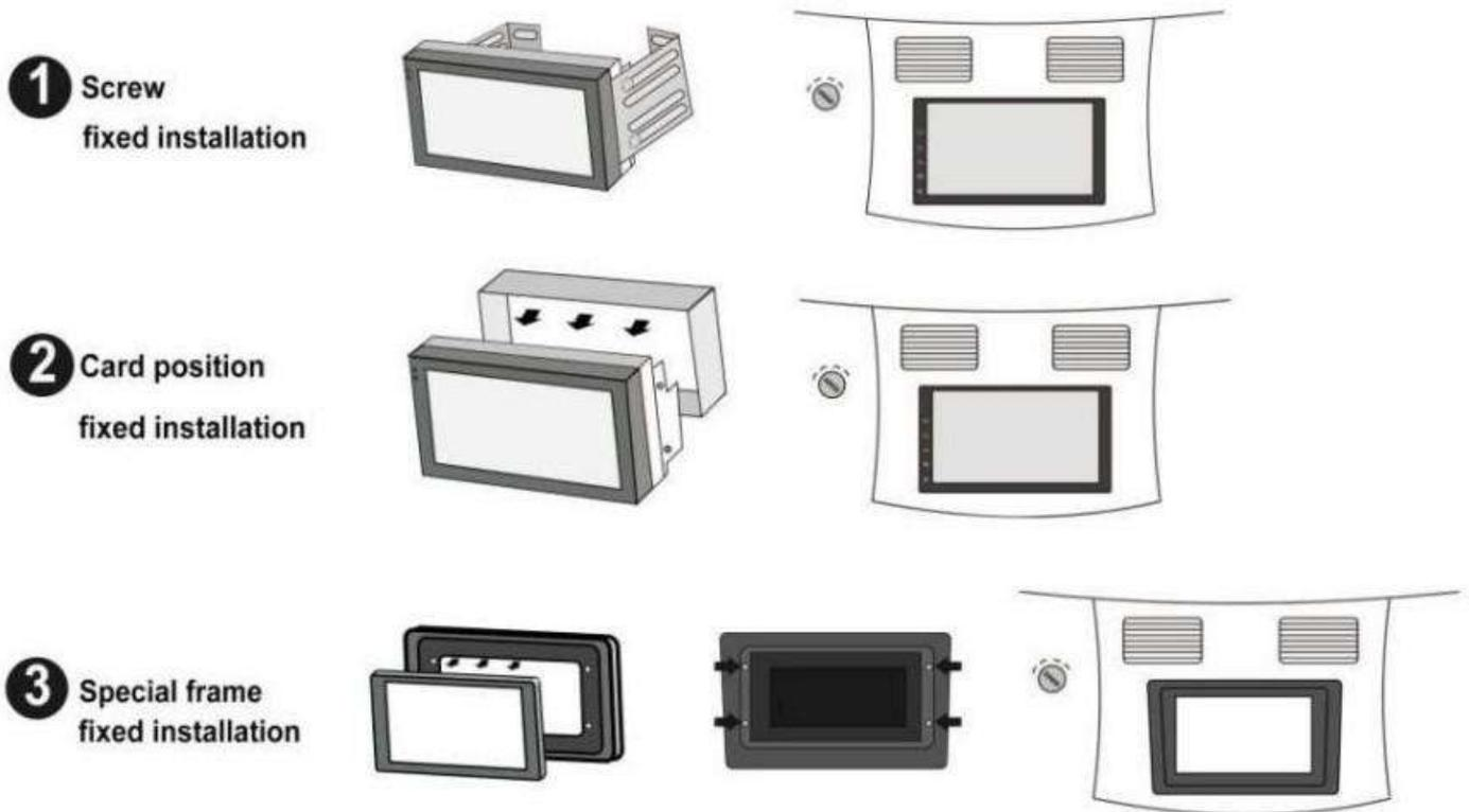
As shown in the figure above, there are three ways to install the machine, please choose one of them according to the actual situation. Of course, you can also re-install the new radio according to the installation method of the original car radio.
