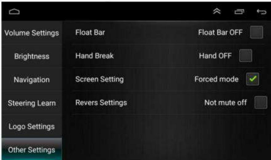
**Float Bar:** press this feature on to have the assitive touch point display on the screen all the time
