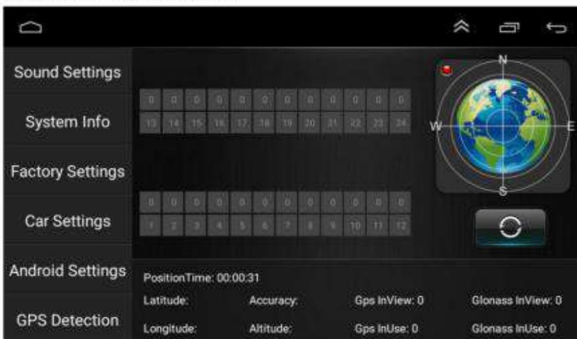
If users can not get the position in the navigation software, users can go here to check the hardware performance. If users can not find the GPS signal, please check if the GPS antenna is placed in the right way, make sure the receiver side is up, the side with stickers is down.
