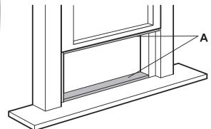
2. Attach the window slider kit to the window stool. Adjust the length of the window slider kit according to the width of window. Cut the adjustable window slider kit if the width of window is less than 67,5 cm.
