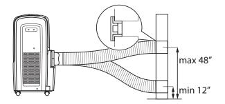
The hose can be extended from its original length of 38,1 cm up to 139,7 cm, but it is the best to keep the length to minimum required. Also make sure that the hose does not have any sharp bends or sags.
