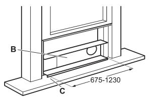
4. Close the window sash securely against the window slider kit.
