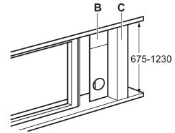
4. Close the sliding sash securely against the window slider kit.
