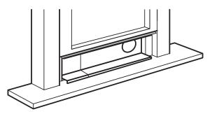
5. Cut the foam seals to an appropriate length and seal the open gap between the top window sash and outer window sash, as shown.
