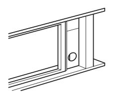
5. Cut the foam seals to an appropriate length and seal the open gap between the sliding sash and outer window sash, as shown.
