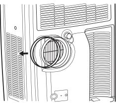
3. Extend either side of the hose and screw the hose to adaptor A.
