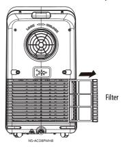
2 Clean the filter with a vacuum cleaner. If the filter is very dirty, it can be washed by hand in warm water with a mild detergent.
