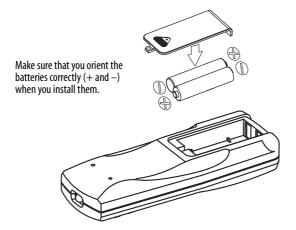
2 Insert three AAA carbon-zinc batteries (provided) into the battery compartment. Note the proper orientation of the + and – polarity of the batteries.
