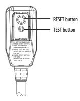
The circuit breaker should be tested periodically by pressing the **TEST** button then the **RESET** button. If the **TEST** button does not cause the circuit breaker to trip, or if the **RESET** button will not stay engaged, unplug the air conditioner immediately and contact an Insignia technician.
