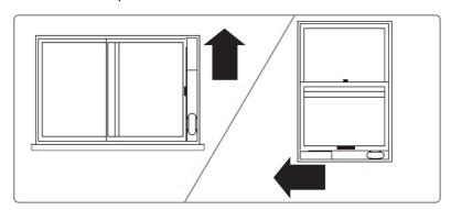
5 Insert the diffuser into the vent panel, then slide it down/left until it clicks into place.
