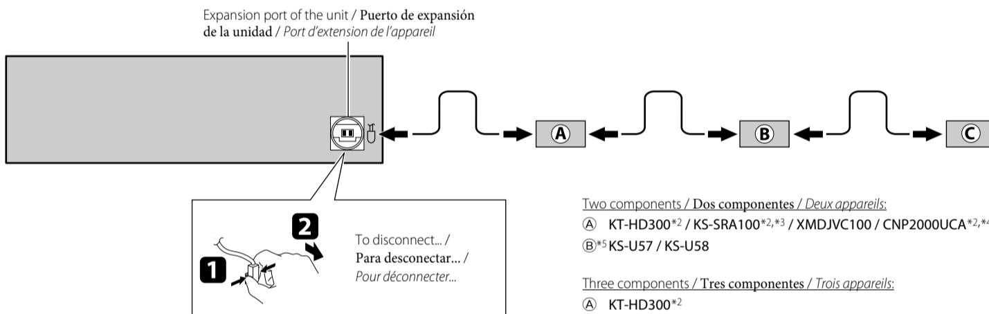
You can connect the HD Radio™ tuner box (KT-HD300) or the following components through the various JVC adapters or system to the expansion port.
