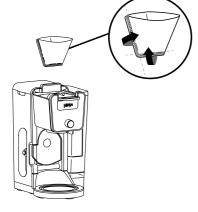
NOTE: Fold the paper filter along the seams, open the top fully, and firmly press it into the brew basket, making sure it is fully seated.
