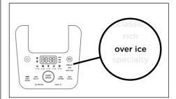
1 Fill your desired vessel to the top with ice cubes and place the vessel below the brew basket. Use the Multi-Serve dial to select the brew size
