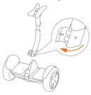
2 Insert the steering bar to the mainframe steering socket
