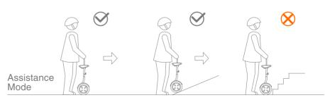
Pull out the draw-bar to enter into the Assistance Mode (automatically when power-on), pushing your Mini flatly may help you move easily under Non-riding mode; please lift the Mini when encountering the stairs, do not push it. Please do as shown on obove.
