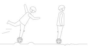
Please keep a moderate speed (3 ~ 10km/h, not Zero/higher speed) with your knees bending when encountering Deceleration zone / threshold,etc,otherwise may cause lost of balance
