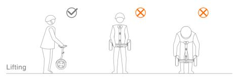
If your Mini is Power ON and in autobalance mode during carrying, power output will be cut off automatically when tires are hung in the air for your safety; balance mode will be recovered automatically when placing Mini to the ground. Do not lift the Mini by the fender or the main frame, or your finger may be clipped or damaged in fender. Please do as shown on above.
