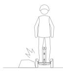
Avoid obstacles contacting the tire rim to cause Mini out of control
