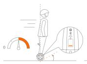
Riding or accelerating when the Mini is alarming or when foot mat tilting up
