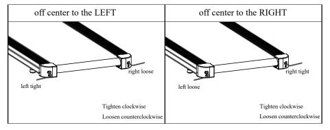
To determine left and right, stand at the rear of the treadmill and face the display Make all belt adjustments on the rear bolt using the hex key provided.
