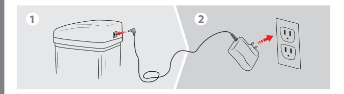
Note: DO NOT operate lid with batteries and AC Adapter at the same time.
