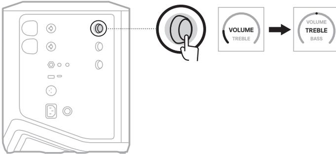
2. Rotate the channel control to either boost or cut the high-frequency balance of the channel.
