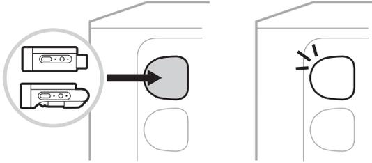
If the system is powered on, on the channel display, a battery icon with a lightning bolt next to it briefly appears to indicate that the transmitter battery is charging. A lightning bolt icon then appears in the upper-right corner of the display. When the transmitter is fully charged, the lightning bolt icon disappears (see page 60).
