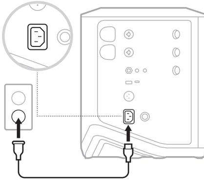
2. Plug the other end of the power cord into an AC (mains) outlet.
