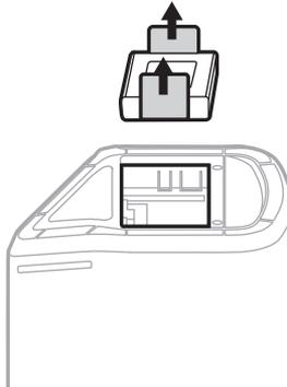
4. Insert the new battery, ensuring the connector pins line up appropriately.
