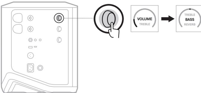
2. Rotate the channel control to either boost or cut the low-frequency balance of the channel.
