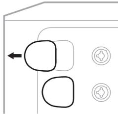
3. Fully insert the transmitter into the charging port until you hear or feel a click, then wait 5 seconds for the transmitter to pair to that channel.
