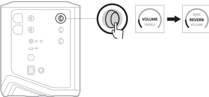
2. Rotate the channel control to adjust the amount of reverb applied to the channel.
