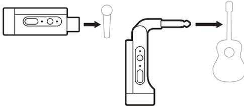
4. Power on the transmitter (see page 39). After a few seconds, a transmitter icon appears on the channel display and the connection light on the transmitter glows solid blue to indicate that the transmitter is connected (see page 63).
