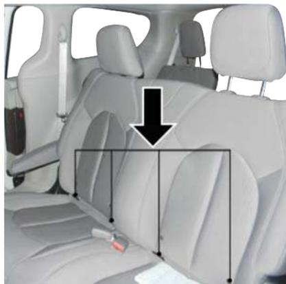
LATCH Anchors (Second Row Bench Anchors Shown) 7 Passenger Bench Seating
