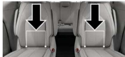
**LATCH Anchorages (Second Row Anchorages Shown) 7 Passenger Stow n' Go Seating**
