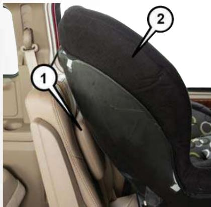
**Car Seat With Head Restraint Folded**
