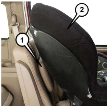
Car Seat With Head Restraint Folded
