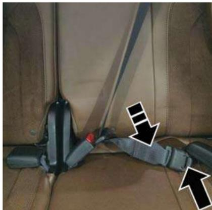
**Mini-Latch And Buckle Connected**
