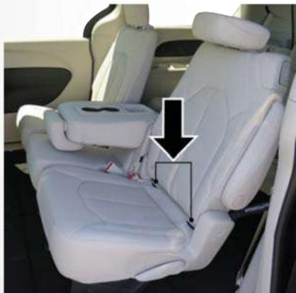
LATCH Anchors (Second Row Anchors Shown) 8 Passenger Seating
