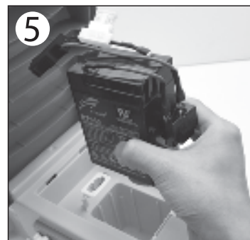
5. Carefully lift the old battery and replace it with a new battery.
