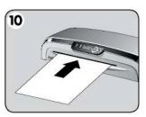
10. Before switching off laminator, feed empty cleaning sheet through machine to clean unit.
