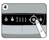
4. Use navigation keys to select setting for the hot lamination pouch thickness (3-7 mil) you wish to laminate.
