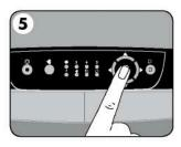
5. Confirm your selection by pressing "Enter" button in the middle of navigation keys. "Wait" LED (S) will begin flashing and laminator will take a few minutes to reach required temperature.
