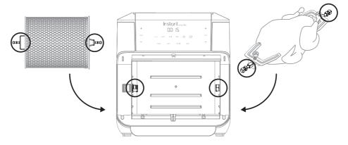
**02** Move the red rotisserie catch lever to the right and hold it in position. Notice that the rotisserie catch inside the cooking chamber withdraws slightly when you move the lever.
