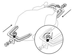
When you're happy with the positioning, tighten the setting screws to hold the forks in place.
