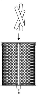
**02** Align the tab on the rotisserie basket with the notch in the lid, then place the lid on the basket.
