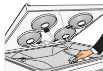
A rod swings up to support the top for cleaning underneath.
