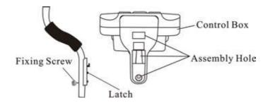
Unscrew the fixing knob on the search coil and remove the knob connector. Place the washers into the groove of the lower stem. Then insert the stem and align the holes on the search coil bracket and the stem. Push the connector through the holes and tighten the knob.
