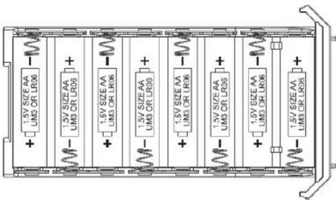
New, Alkaline or Lithium, 'AA' batteries must be inserted with the orientation as shown on the tray. As with most electronic devices the negative ( - ) orientation of the batteries should be against the springs. Failure to insert the batteries properly will cause damage to the unit.
