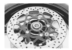
• Remove the brake discs, left and right.
