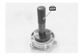
· Remove the driveshaft left bearing dust seal from the retainer using the special tool.
