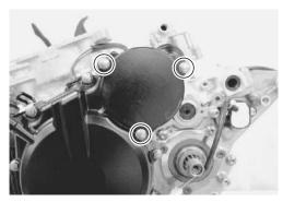
• Remove the spring washer ①, washer ② and starter idle gear No. 1 ③.
