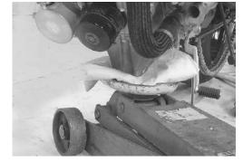
• Remove the engine mounting bolt (A).
