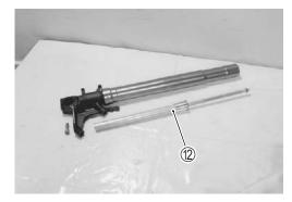
• Slide the outer tube to remove it from the inner tube.
