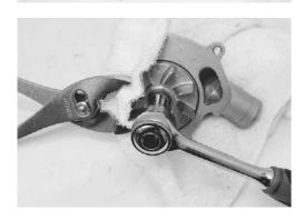
• Remove the mechanical seal ring ④ and rubber seal ⑤ from the impeller.
