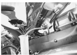
• Disconnect the fuel pump lead wire coupler 3.
