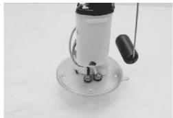
• Remove the lead wire ①, screws and fuel level gauge ②.
