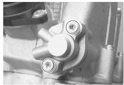
Turn the crankshaft approx. 180° counterclockwise to make the push rod come out from the adjuster against the cam chain, via chain tensioner.
