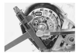
• Lock the clutch sleeve hub nut with a center punch.
