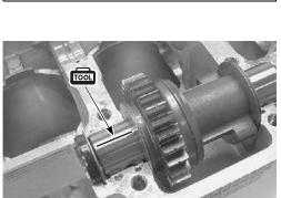
Remove the middle crankcase and measure the width of the compressed plastigauge using the envelope scale. This measurement should be taken at the widest part of the compressed plastigauge.
