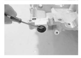
• Remove the gearshift shaft bearings with the special tool.
