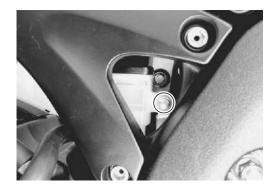
• Loosen the rear shock absorber bracket.
