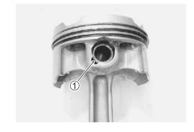
• Separate the piston and conrod by driving out the piston pin.
