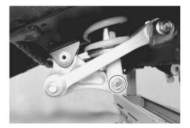
• Remove the rear shock absorber.
