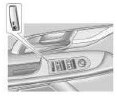
Press the button on the driver door armrest to activate the safety locks on the passenger rear doors.
