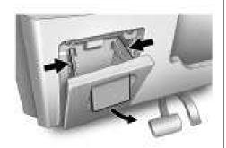
The instrument panel fuse block is located in the instrument panel, on the driver side of the vehicle. To access the fuses, open the fuse panel door by pulling down at the top.
