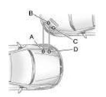
Connect one end of the red positive (+) cable to the jump start positive (+) post (A). Use a remote positive (+) terminal if the vehicle has one.
