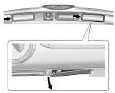
2. Push the end on either of the lamp assemblies (passenger side shown) and then move the lamp assembly down to remove it from trunk lid.
