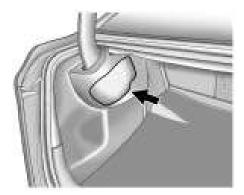
The rear compartment fuse block is located on the left side of the trunk behind a cover.
