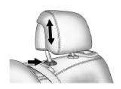
Pull the head rest up to raise it. To lower the head rest, press the release button, located on the head rest post on the top of the seatback, while you push the head rest down.
