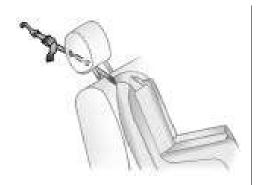
If the position you are using has an adjustable headrest or head restraint and you are using a single tether, route the tether under the headrest or head restraint and in between the headrest or head restraint posts. See *Head Restraints* on page 2-2.
