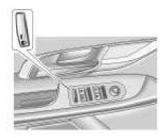
The power window switches located on the driver door control all four windows. The passenger door only has a window switch that controls that window. Push the switch down to open the window. Pull the front of the switch up to close it.
