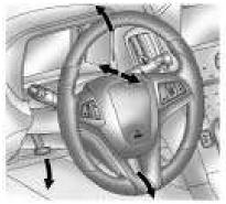
The adjustment lever is located on the left side of the steering column.
