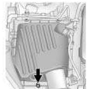
Remove the screws on top of the engine air cleaner/filter housing.
