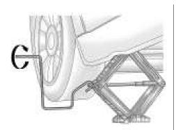
Turn the jack handle clockwise to raise the vehicle far enough off the ground for the compact spare to fit under the vehicle.
