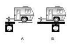
The trailer tongue (A) should weigh 10-15 percent of the total loaded trailer weight (B).
