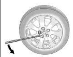
3. Turn the wheel wrench counterclockwise to loosen all the wheel nuts, but do not remove them yet.
