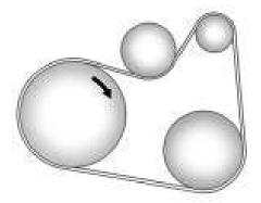
2.4L L4 Engine (Electric Power Steering)
