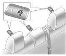
The top tether anchors are located under the covers, behind the rear seat, on the filler panel. Be sure to use an anchor located on the same side of the vehicle as the seating position where the child restraint will be placed.
