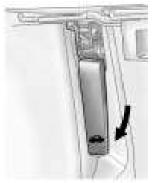
Pull the interior hood release handle located to the left of the steering column below the instrument panel.
