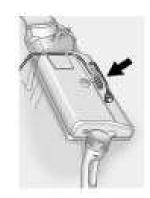
The electrical cord is located on the driver side of the engine compartment, between the fender and the engine compartment fuse block.
