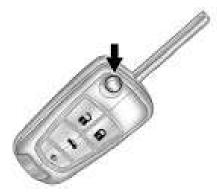
Press the button on the RKE transmitter to extend the key. Press the button and the key blade to retract the key.
