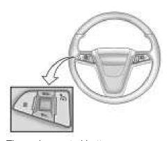
The cruise control buttons are located on the steering wheel.
