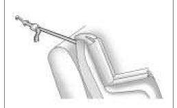
If the position you are using does not have a headrest or head restraint and you are using a single tether, route the tether over the seatback.
