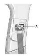
Press the release button (A) and move the height adjuster to the desired position. The adjuster can be moved up by pushing the slide/ trim up. After the adjuster is set to the desired position, try to move it down without pushing the release button to make sure it has locked into position.
