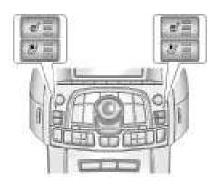
On vehicle with the heated and ventilated cooled seat feature the buttons are located near the climate controls.
