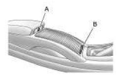
A two tiered storage area is under the front adjustable armrest. Push the button (A) on the underside of the front edge of the cover to open.
