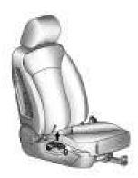
On vehicles with manual reclining seatbacks, the control lever is located on the outboard side of the seat.
