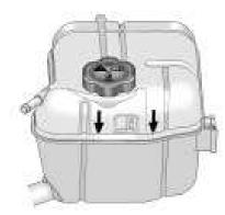
3. Fill the coolant surge tank with the proper mixture to the mark pointed to on the front of the coolant surge tank.
