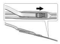
Lift up on plastic latch in the middle of the wiper blade where the wiper arm attaches.
