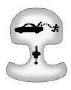
There is an emergency trunk release handle located inside the trunk on the trunk latch. On some vehicles, the release handle can be accessed by folding the rear seat center seatback. See *Rear Seats on page 2-9*. Pull the release handle to open the trunk from the inside.
