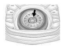
3. Turn the retainer nut counterclockwise and remove the spare tire.
