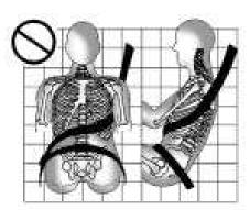
A: The shoulder belt is worn under the arm. It should be worn over the shoulder at all times.
