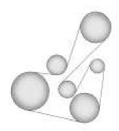
2.4L L4 Engine (Hydraulic Power Steering)
