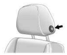
To raise or lower the head restraint, press the release button located on the side of the head restraint and pull up or push the head restraint down and release the button.
