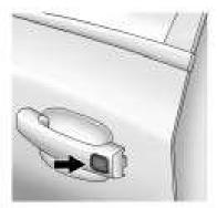
When all doors are closed and the ignition is off, the vehicle can be locked by pressing this area on the door handle. This feature will be available for several minutes after the vehicle has been turned off.
