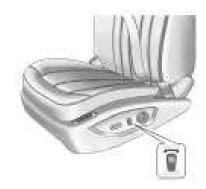
On vehicles with power reclining seatbacks the vertical control is located on the outboard side of the seat.
