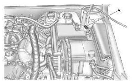
Check the other vehicle. It must have a 12-volt battery with a negative ground system.
