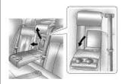
The vehicle has a small door in the rear seat. This door allows access to the trunk from inside the vehicle.
