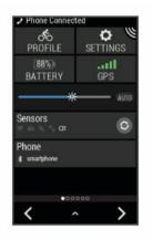
The settings widget appears. A flashing icon means the device is searching for a signal. A solid icon means the signal was found or the sensor is connected. You can select any icon to change the settings.
