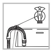
If it is placed over the edge of a basin or sink be sure the free end of the hose should not be underwater.
