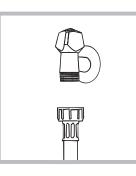
1. Connect the supply pipe by screwing it to a cold water tap using a <sup>3</sup>/<sub>4</sub> gas threaded connection (see figure).
