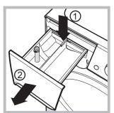
To remove the drawer, press lever (1) and pull the drawer outwards (2) (see figure). Wash it under running water; this procedure
