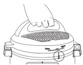
**02** Turn the lid clockwise until the ▼ on the lid aligns with the middle of the control panel.
