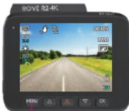
Then Press and hold the **MENU** button again to switch from Photo mode to Playback mode
