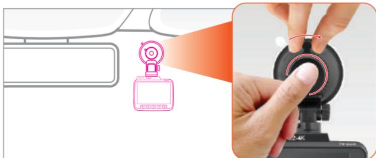
*Press the suction mount against windshield and while pressing, turn the LOCKING Knob towards LOCK position to lock the mount in place.*
