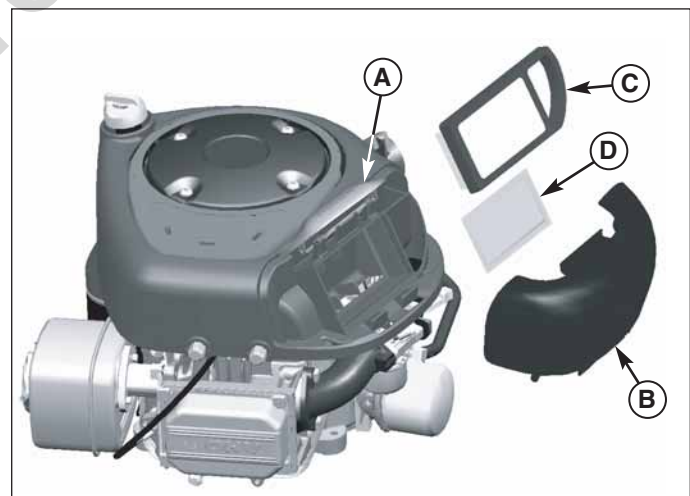
Figure 30. Air Filter Service - Briggs & Stratton Single Cylinder Models A. Air Filter Latch B. Air Filter Cover C. Air Filter D. Pre-Cleaner
