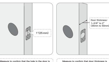
Measure to confirm that the hole in the door is
