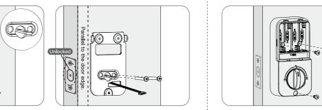
Secure the interior assembly with the supplied screws.
