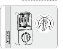
Test the lock by rotating the thumb turn to see if the bolt can be extended and retracted
