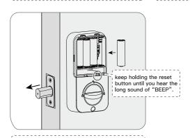
Keep holding the reset button, and load the last battery. Hold the reset button until you hear the long sound of "BEEP". The lock will automatically go into locking position. This is for the smart lock to memorize the orientation of the door.
