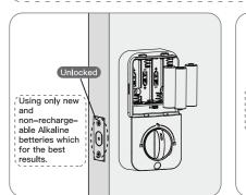
While the door is open and unlock, load 3AA batteries into the interior assembly.
