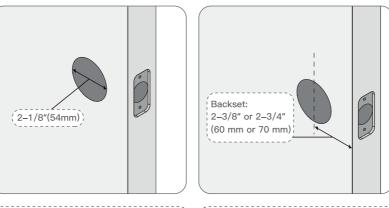
Measure to confirm that the hole in the door is 2-1/8"(54mm).
