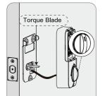
Rotate the Thumb turn in vertical position and insert the horizontal orientation of torque blade into the interior assembly lock switch.
