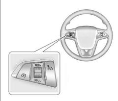
ress to turn the cruise control system on and off. A white indicator light will turn on or off in the instrument cluster.
