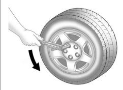
4. Turn the wheel wrench counterclockwise to loosen all the wheel nuts, but do not remove them yet.
