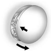
The fuel cap is behind the fuel door on the vehicle's passenger side. To open the fuel door, push the rearward center edge in and release.
