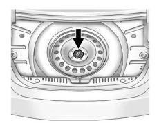
3. Turn the retainer nut counterclockwise and remove the spare tire. Place the spare tire next to the tire being changed.
