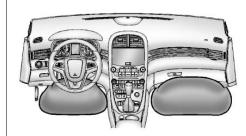
The driver knee airbag is below the steering column. The front outboard passenger knee airbag is below the glove box.
