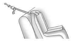
If the position you are using does not have a headrest or head restraint and you are using a single tether, route the tether over the seatback.
