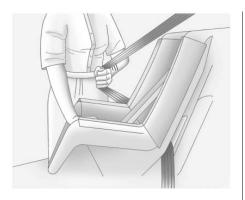
4. Pull the shoulder belt all the way out of the retractor to set the lock. When the retractor lock is set, the belt can be tightened but not pulled out of the retractor.
