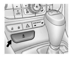
To turn the system off, press the TCS/StabiliTrak button on the center stack.
