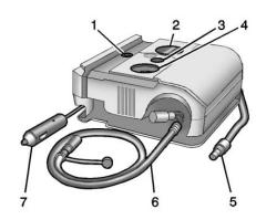
When using the tire sealant and compressor kit during cold temperatures, warm the kit in a heated environment for five minutes. This will help to inflate the tire faster.
