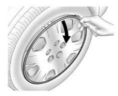
Take off the wheel cover or center cap, if the vehicle has one, to reach the wheel bolts.
