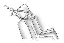
If the position you are using has an adjustable headrest or head restraint and you are using a dual tether route the tether around the headrest or head restraint. 3. Before placing a child in the child restraint, make sure it is securely held in place. To check, grasp the child restraint at the LATCH path and attempt to move it side to side and back and forth. There should be no more than 2.5 cm (1 in) of movement for proper installation.
