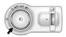
The exterior lamp control is on the instrument panel on the left side of the steering wheel.
