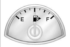
When the ignition is on, the fuel gauge shows how much fuel is left in the fuel tank. When the indicator nears empty, a message in the Driver Information Center (DIC) displays. See *Fuel System Messages on page 5-32*. The vehicle still has a little fuel left, but the vehicle should be fueled soon.
