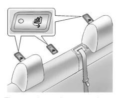
The top tether anchors are under the covers, behind the rear seat, on the filler panel. Be sure to use an anchor on the same side of the vehicle as the seating position where the child restraint will be placed.
