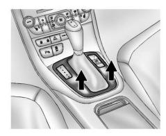
Release the shift lever trim from the center console at the rear, then fold upward and turn it to the left.
