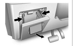
The instrument panel fuse block is in the instrument panel, on the driver side of the vehicle. To access the fuses, open the fuse panel door by pulling down at the top.
