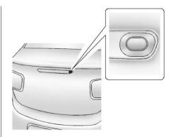
Unlock the trunk first by pressing on the center stack, front door panel, or RKE transmitter. Then, press the touch pad on the trunk Center High-Mounted Stoplamp (CHMSL).
