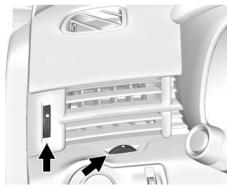
Use the thumbwheels to change the direction of the airflow.
