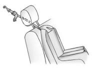
If the position you are using has an adjustable headrest or head restraint and you are using a single tether, route the tether under the headrest or head restraint and in between the headrest or head restraint posts.
