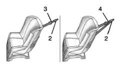
A top tether (3, 4) anchors the top of the child restraint to the vehicle. A top tether anchor is built into the vehicle. The top tether attachment (2) on the child restraint connects to the top tether anchor in the vehicle in order to reduce the forward movement and rotation of the child restraint during driving or in a crash.
