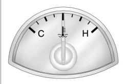
This gauge shows the engine coolant temperature.
