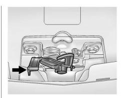
Go to the front of the vehicle and push the secondary hood release handle toward the driver side of the vehicle.
