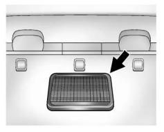
The eAssist system high voltage battery is cooled with air drawn from the vehicle interior. The cold air intake for the battery is behind the rear seat, on the filler panel. Do not cover the intake.
