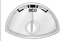
For eAssist vehicles, this gauge assists in driving efficiently and will vary based on driver input.
