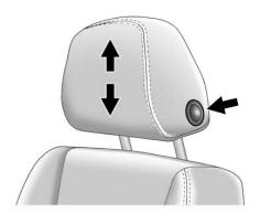
To raise or lower the head restraint, press the button located on the side of the head restraint and pull up or push the head restraint down and release the button.
