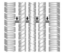
Treadwear indicators are one way to tell when it is time for new tires. Treadwear indicators appear when the tires have only 1.6 mm (1/16 in) or less of tread remaining. See *Tire Inspection on page 10-59* and *Tire Rotation on page 10-59*.
