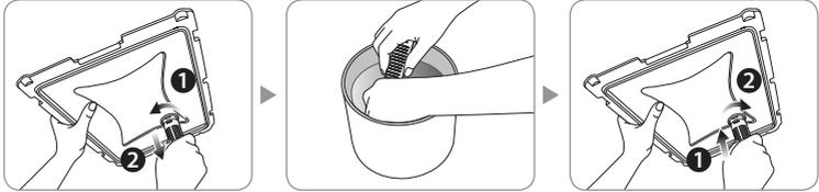
6. Wipe the inside of water tank with a clean soft cloth.
