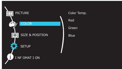
Press menu enter setting. Then press down to scroll and choose "COLOR". Double press enter color setting. You can adjust "Red" "Green" "Blue" to press up or down.
