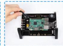
5 Mount the raspberry pi with a screwdriver on the back of the monitor.
