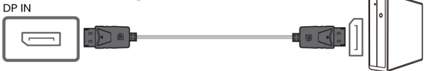
— A DP cable shorter under 1.5 m in length is recommended. Using a cable longer than 1.5 m can affect the picture quality.
