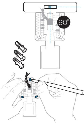
**12 Set R-switch position and insert R-wire or wires.**
