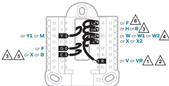
**NOTE:** Do **NOT** use **W** for heat pump applications. Auxiliary heat must wire to **AUX** or **E**.
