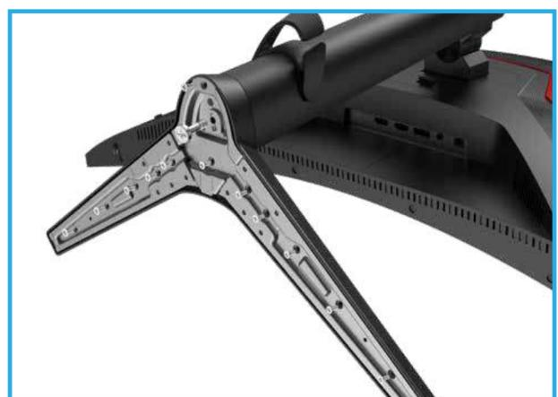
As shown, turn the screw in the direction of the arrow to remove the bracket neck from the bracket base.
