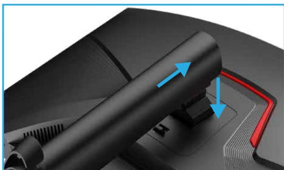
Push the column into the main body of the monitor in the direction indicated by the arrow; Check whether the bracket and the main body are firmly connected;
