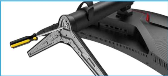
Use 2# cross screwdriver to tighten the screws clockwise.
