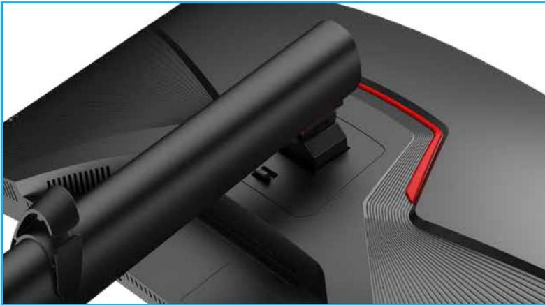
Place the foamed polystyrene (Mat) in the package on the floor and place the product face down on the foamed polystyrene as shown. If you don't have styrofoam, use a thick cushion.
