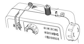
As shown in the drawing, the thread passes through the bobbin hole, and is winded 3-4 times to the right around the bobbin.
