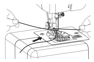
Pass the upper and bobbin threads to the rear under the presser foot, pulling them out together about 10 cm.
