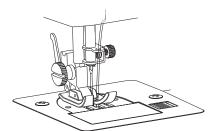
Rotate the hand wheel to raise the needle to its highest position and pass the thread through the eye of the needle from the front.
