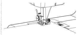
6 Lower the presser foot lifter to fasten the fabric.
