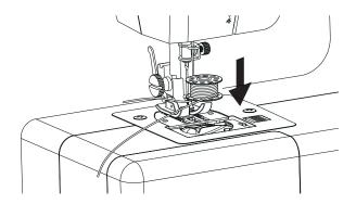
Hold the end of the upper thread and rotate the hand wheel toward you (counterclockwise) while gently pulling on the upper thread until the bobbin thread emerges from the bobbin thread hole.
