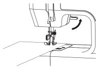
When you use the sewing machine for the first time, remove the test piece (this is a piece of fabric used for test sewing when the machine is shipped from the factory).
