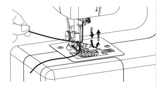
Pull the bobbin thread when it emerges from the bobbin thread hole. It's easier to pull the thread out if you use a rod with a small tip.
