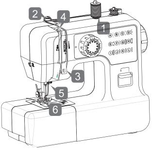
Pass the thread through the upper thread guides. Through the groove
