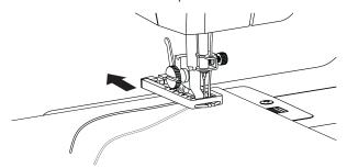
Draw both of needle and bobbin thread to the left. Slider frame of buttonhole is removable. Move the slider frame toward you so that the top mark on the slider meets the start mark.
