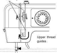
Pass thread through the take-up lever. When the take-up lever is in its lowest position, rotate the hand wheel to its highest position.
