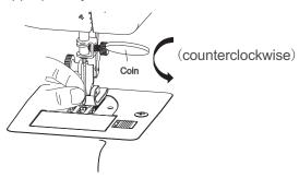
Insert a new needle in the needle clamp so that the flat part faces the back, turn the needle clamp screw clockwise, and tighten the needle in place.
