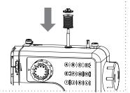
Place the thread through the thread tension disk and pass the thread through the groove.
