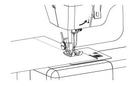
Turn the pattern selection dial to align with the mark indicating the desired stitch.
