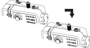
Move the switch to "I " or "II" to start winding the bobbin
