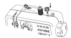
Slide the bobbin winding spindle to the right.
