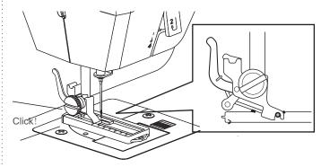
Raise the presser foot lifter, pass the upper thread and the bobbin thread through the buttonhole presser foot so they come out from the side.
