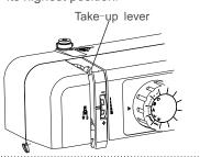
Turn the hand wheel to bring the take-up lever to its lowest position and pass the thread through the thread guide.
