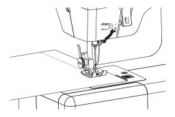
Remove the fabric and cut the thread with the thread cutter.
