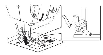
Raise the presser foot lock lever to secure the presser foot to the presser holder.
