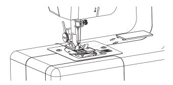
Pull out about 10 cm of thread from the bobbin and insert the bobbin so it winds to the right.
