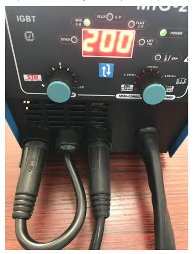
Step.6-Clamp the ground clip to the workpiece, then start your MIG work.
