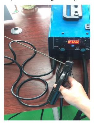
Step.4- Clamp the ground clamp to the workpiece.
