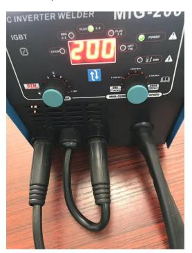
Step.5-Clamp the ground clip to the workpiece, then start your MIG work.
