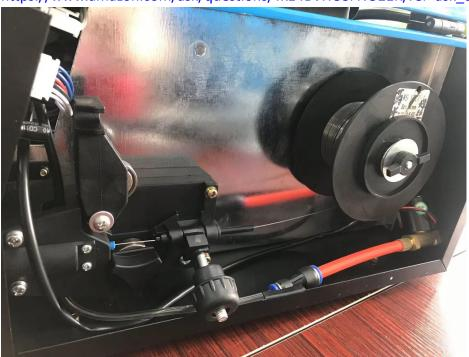
\*Connect the welding wire to the wire feeding device, pay attention to insert the welding wire directly into the wire guide tube, and then press the welding wire well.
