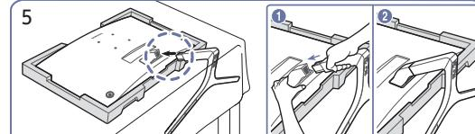
Hold the back of the monitor as shown in the figure.
