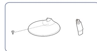
Tightly fasten the connecting screw at the bottom of the stand base.
