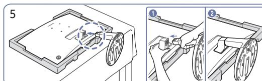
Hold the back of the monitor as shown in the figure.
