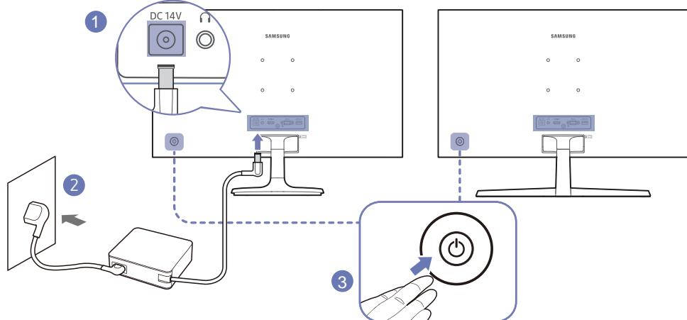
1 Connect the power cable to the AC/DC adapter. Then, connect the AC/DC adapter to the DC14V port on the back of the product.
