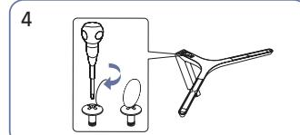
Tightly fasten the connecting screw at the bottom of the stand base.
