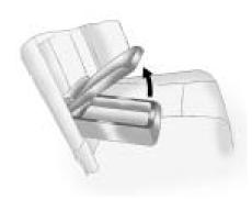
To access the rear seat armrest, pull the handle down. Lift the top of the armrest to access the storage area.
