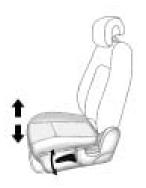
If the vehicle has a manual driver seat height adjuster, it is located on the outboard side of the seat near the front of the seat cushion.
