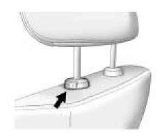
Pull the head restraint up to raise it. To lower the head restraint, press the button, located on the top of the seatback, and push the restraint down. Push down on the head restraint after the button is released to make sure that it is locked in place.
