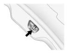
To open the liftgate if the vehicle's battery is disconnected or the voltage is low, access the release lever. Remove the interior trim cover on the inside of the liftgate. Use a tool to push the lever on the latch until the liftgate releases.
