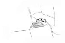
2. Lift the lever located on the top of the seatback to release the seatback and fold the seatback forward.
