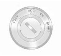
The ignition switch has four different positions.
