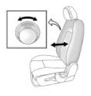
If the vehicle has this feature, the knob is located on the inboard side of the driver seatback.
