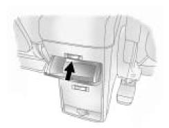
To open the cover of the rear storage area, push the button located at the top.
