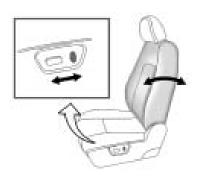
If the seats have power reclining seatbacks, the control used to recline them is located on the outboard side of the seat.
