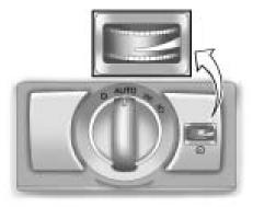
The thumbwheel for this feature is located on the left side of the steering wheel next to the exterior lamps control.
