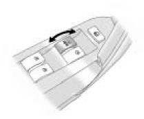
The window switches for all doors are located on the driver door. Each door also has a switch.
