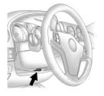
The tilt lever is located on the left side of the steering column.
