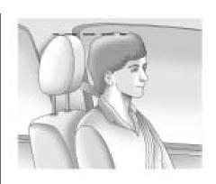
Adjust the head restraint so that the top of the restraint is at the same height as the top of the occupant's head. This position reduces the chance of a neck injury in a crash.
