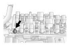
Your vehicle is equipped with a remote positive (+) terminal. This is located in the engine compartment on the driver side of the vehicle, on the underhood fuse block. See *Engine Compartment Overview on page 5-12* for more information on location. To uncover the remote positive (+) terminal, press the tab on the bottom of the fuse block and lift the cover up.
