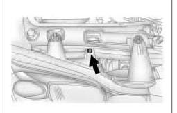
Locate the vertical headlamp aiming screws, which are under the hood near each headlamp assembly.
