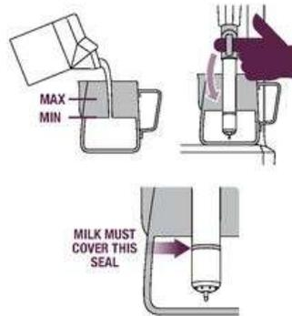
To start, press down and release steam lever. The LCD will display the temperature of the milk as it heats. Milk texturing will stop automatically when the selected milk temperature is reached. Lift steam wand to remove milk jug. **Wipe the wand & tip with a damp cloth.** Lower steam wand to the down position and the wand will automatically purge.
