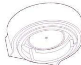
7. Re-insert the dispersion plate, then the shower screen, then the screw. With your fingers, turn the screw clockwise for 2-3 revolutions then insert the Allen Key to tighten until the screw is flush with the shower screen. Do not overtighten screw.
