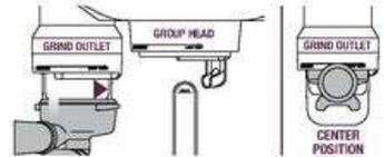
To start the auto grind, dose & tamp function, rotate the portafilter to the right then gently guide back to the center position. Grinding will commence.
