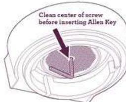
5. Once loosened, carefully remove and retain the screw, stainless steel shower screen and black dispersion plate. Make note of the side of the shower screen and dispersion plate that are facing downwards. This will make re-assembly easier. Wash the shower screen and dispersion plate in warm soapy water, then dry thoroughly.
