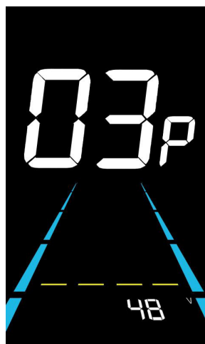
Rated voltage setting interface
