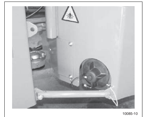
Articulated frame steering blocking device latched
