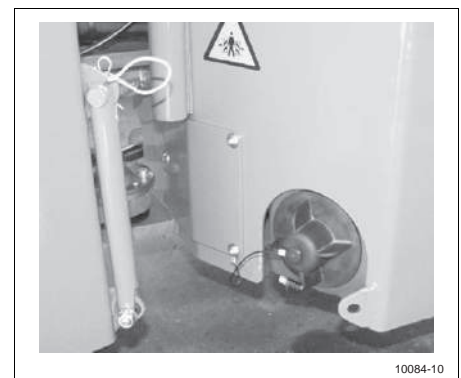
Articulated frame steering blocking device released
