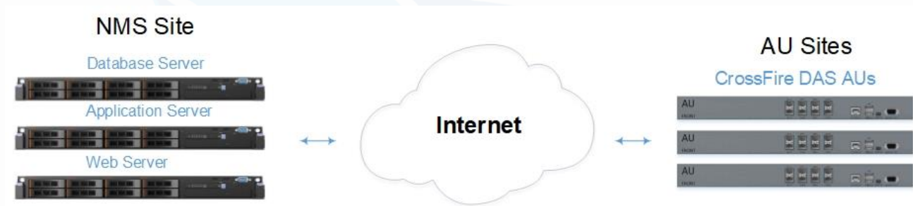
Figure 15. NMS System Architecture
