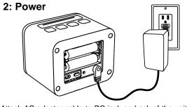
Attach AC adaptor cable to DC jack on back of the unit and plug the other end into a wall socket.
