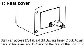
Staff can access DST (Daylight Saving Time), Clock Adjust, backup batteries and DC jack on the rear of the unit. Turn the thumbscrew to remove the Rear Cover. Replace Rear Cover after adjusting settings.
