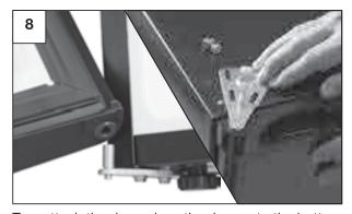
To reattach the door, place the door onto the bottom axle insert. Place the top **bracket** into the door and align the metal **bracket** holes over the holes in the top of the refrigerator cabinet. Tighten the two screws to hold in place.
