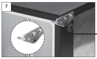
With the unit on its side, remove the bottom metal **base bracket**. Then gently place the refrigerator on opposite side to complete the door reversal.
