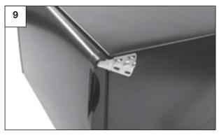
The rubber gasket should be compressed on all sides of the door. If the gasket is more compressed on one side, the metal bracket position should be adjusted. Once the door position is finalized, securely tighten the screws.
