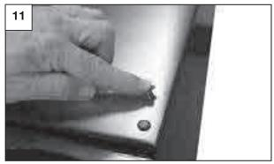
Reinstall all plastic **hole insert plugs**. The reinstallation of the plastic **hole insert plugs** is important to maintain the seal and integrity of the insulation.
