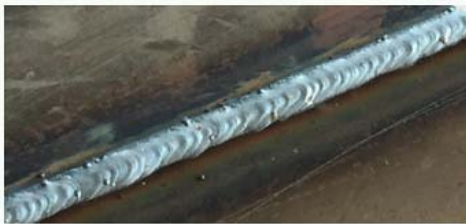
4mm carbon steel plate angle welding performing
