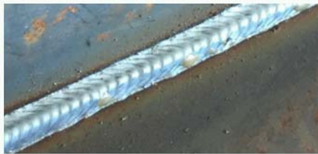
220V 6mm steel plate angle welding
