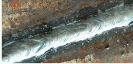
Ø3.2 & Ø4.0mm electrode thickness 5mm flat welding
