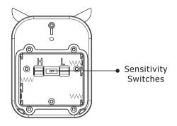
**Step 3** Insert the 3pcs AA 1.5V Alkaline Batteries and note the anode and cathode (Batteries are not included).
