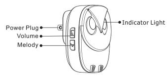
Power Plug:plug the receiver into an outlet.
