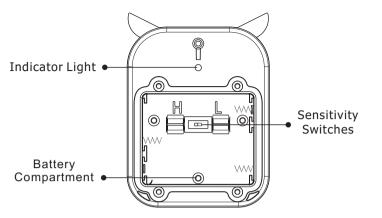
**Indicator Light:** flashes once meaning the motion sensor was activated and sent the wireless signal.
