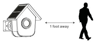
(The indicator of the ON/OFF button will flash for once, indicating that the motion sensor has been activated and has sent the wireless signal; then the motion sensor will be automatically reset a few seconds later, ready for the next trigger)
