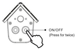
(The indicator of the ON/OFF button will flash for once, indicating that the motion sensor has been activated and has sent the wireless signal)
