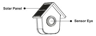
**Solar Panel:** charge the built-in battery of the sensor **Sensor Eye:** it detects heat movements
