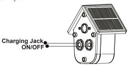
**Charging Jack:** Pull out the red plug and connect the additional solar panel or DC 5V power adapter
